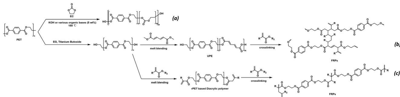
**Fig. 5** (a) Synthesis of polyols via reaction of EC with waste PET. (b) Synthesis of FRPs through crosslinking of UPE obtained via glycolysis of PET followed by the reaction with olefinic diacids. (c) Synthesis of FRPs through crosslinking of the PET-based diacrylic polymer synthesized via glycolysis of PET followed by the reaction with olefinic monoacids.
