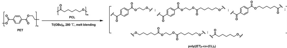
**Fig. 10** Synthesis of poly((ET)<sub>x</sub>-co-(CL)<sub>y</sub>) via transesterification of PET and PCL through melt blending.
