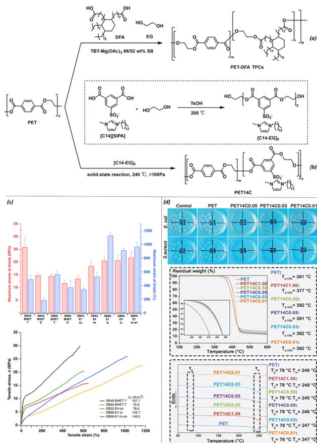
**Fig. 8** (a) One-pot upcycling of rPET into segmented TPCs using the renewable DFA as the soft building block. (b) Upcycling of PET into antibacterial PET14C using the [C14-EG]<sub>5</sub> oligomer. (c) Mechanical properties and stress–strain curves of TPCs. Reproduced from ref. 43 with permission from American Chemical Society, copyright 2022. (d) Antibacterial and thermal properties of the recycled PET14C. Reproduced from ref. 52 with permission from John Wiley and Sons, copyright 2023.
