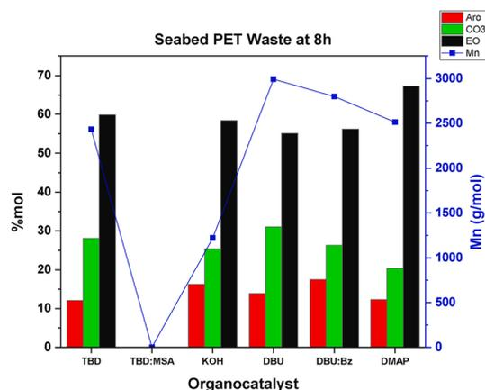
**Fig. 6** Chemical composition and molecular weight of polyols derived from PET waste within 8 h using varying basic organocatalysts and KOH. Reproduced from ref. 44 with permission from Elsevier, copyright 2024.
