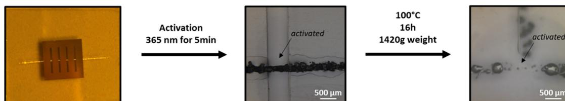
**Fig. 7** Photopatterned-healing experiment of a cut in a cured film using a photomask. The healing of the cut is achieved by using 365 nm UV light to activate the **TMG-NOA**, followed by exposure to an elevated temperature of 100 °C and a 1420 g weight for 16 hours. The activated part is marked with an arrow.
