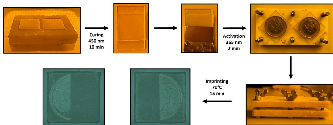
Fig. 5 Imprinting experiment with cured films at 450 nm. One sided spatial activation of the photolabile base **TMG-NOA** was induced with 365 nm UV-light and imprinting of the 1-euro coins was performed by using a Teflon press at 70 °C for 15 minutes.
