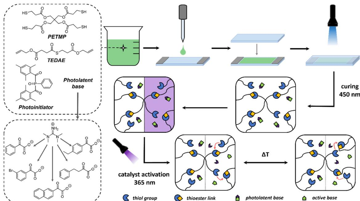
**Fig. 1** General scheme for the manufacturing process of the dynamic thiol-ene network: curing of the formulation between two glass slides using 450 nm UV-light followed by a spatial activation (365 nm UV-light) of the photolatent base and thermally activated thiol-thioester exchange.
