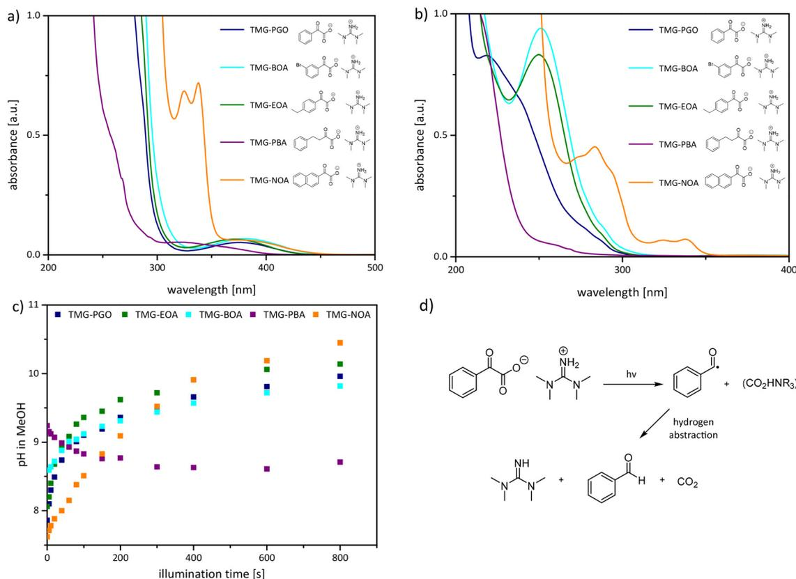
**Fig. 2** (a) UV-Vis absorption spectra of TMG-PLBs  $1 \times 10^{-3}$  mol L<sup>-1</sup> in acetonitrile. (b) UV-Vis absorption spectra of TMG-PLBs  $1 \times 10^{-4}$  mol L<sup>-1</sup> in acetonitrile. (c) pH measurements of TMG-PLBs in methanol ( $0.06$  mol L<sup>-1</sup>) upon irradiation with 365 nm UV-light. (d) Activation mechanism of the TMG-PLB with **TMG-PGO** as example.<sup>25</sup>
