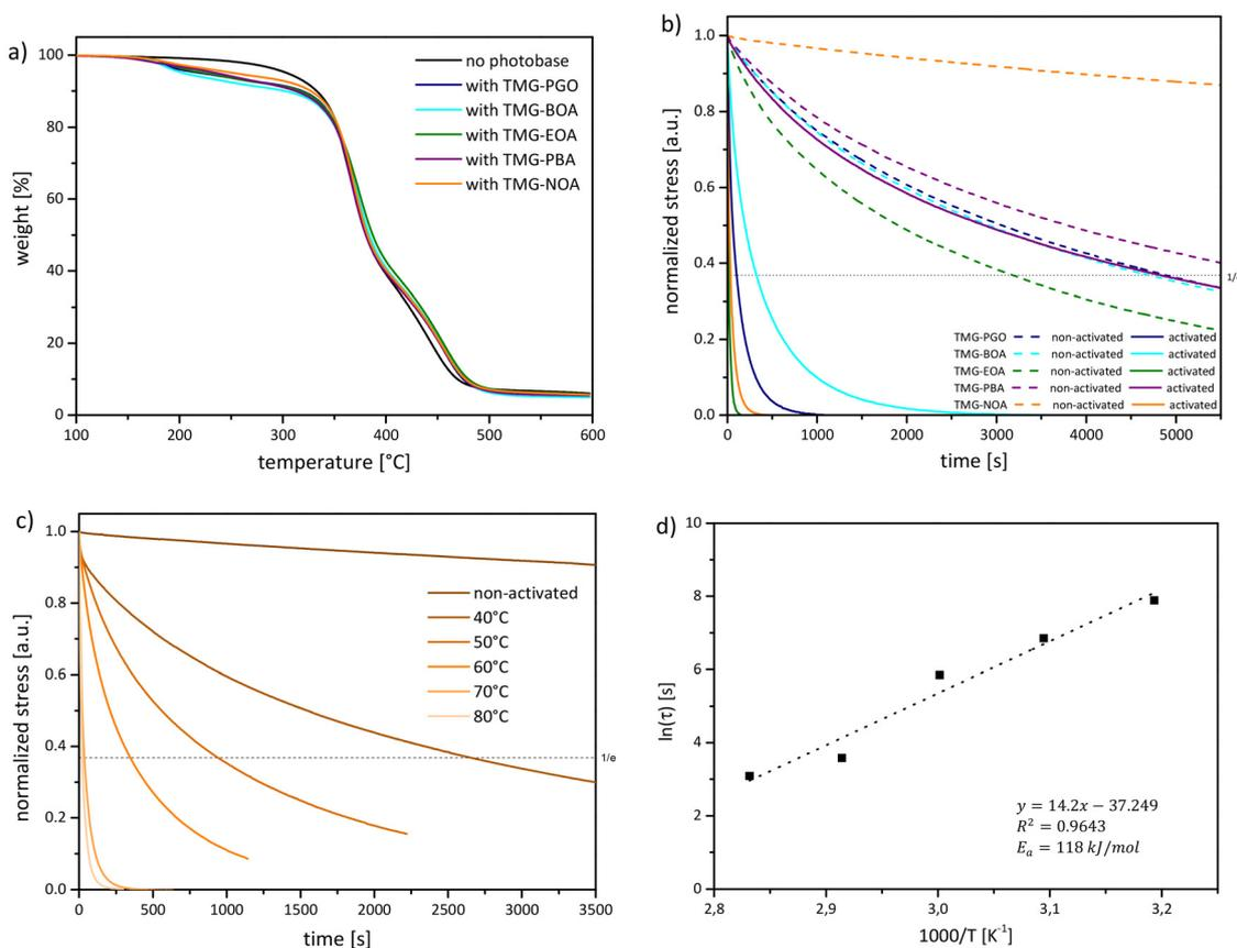
**Fig. 4** (a) Thermogravimetric analysis of the cured photopolymer with incorporated TMG-PLBs. (b) Normalized stress relaxation curves of the activated and non-activated networks containing the TMG-PLBs at 70 °C. (c) Normalized stress relaxation curves of the activated network containing TMG-NOA at a temperature range of 40 °C–80 °C. (d) Arrhenius plot of the network containing TMG-NOA.
