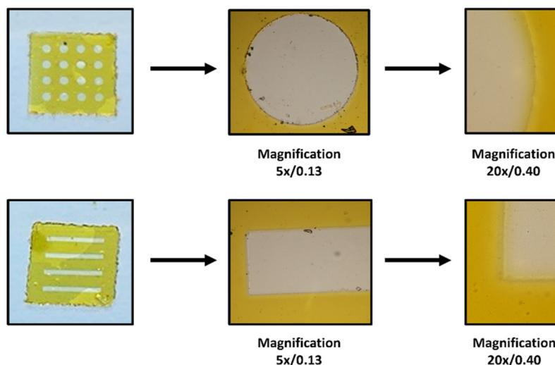
**Fig. 6** Photochemical drawing on a cured film (10 mm × 10 mm) using 365 nm UV-light and a photomask (lined/dotted). Microscopic images with magnifications of 5x/0.13 and 20x/0.40 are presented for both films.
