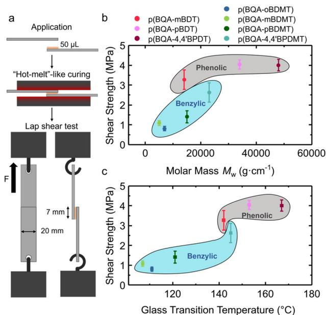
**Fig. 5** Performance analysis and testing of seven TCC adhesives by bonding aluminium substrates. Schematic lap shear test setup (a) and global property correlation plots comparing adhesive strength with  $M_{w,app}$  (b) and  $T_g$  (c). (Data points represent the average. Error bars indicate the standard deviation of the tested samples with  $n = 6$  and the background colour in b & c is only to guide the eye.)
