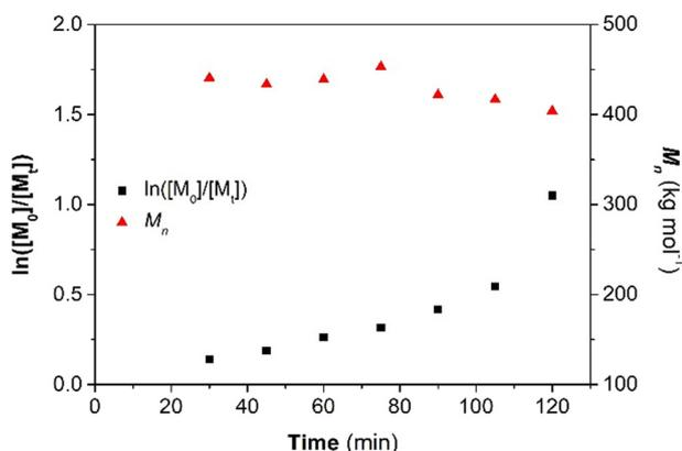
Fig. 2 Fe(acac)<sub>3</sub> mediated conventional polymerization of MA at different polymerization time performed at MA/Fe/Si–H = 200/0.5/0.25.
