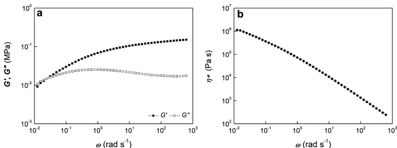
Fig. 4 (a) Shear storage and loss modulus and (b) complex viscosity as a function of angular frequency of entry 6.
