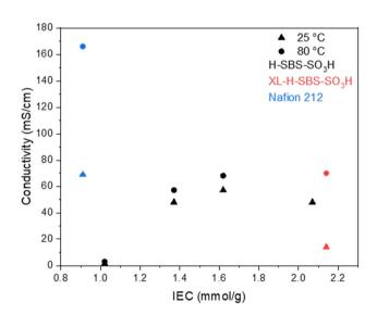
Fig. 8 Conductivity at 25 °C (circle) and 80 °C (triangle) of H-SBS-SO<sub>3</sub>H (black), XL-H-SBS-SO<sub>3</sub>H-2.14 (red) and Nafion 212 (blue).
