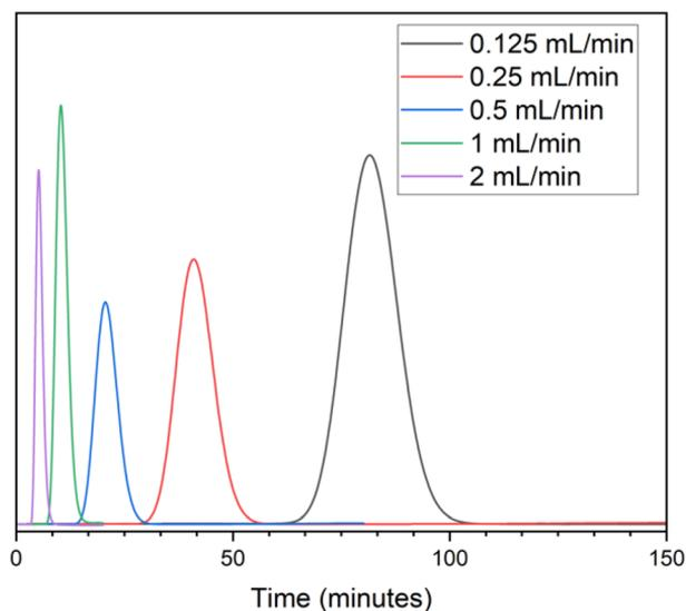
Fig. 5 Raw RTD traces of toluene in a 10 mL reactor at flow rates 2 mL min<sup>-1</sup> to 0.125 mL min<sup>-1</sup>.
