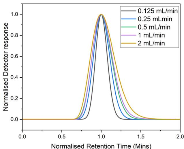
Fig. 6 Normalized RTD traces of toluene in a 10 mL reactor at flow rates 2 mL min<sup>-1</sup> to 0.125 mL min<sup>-1</sup>.
