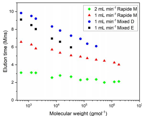
Fig. 3 Overlaid calibration samples using a Rapide M at 1 and 2 mL min<sup>-1</sup> and Agilent mixed E and D columns at a pumping speed = 1 mL min<sup>-1</sup>.
