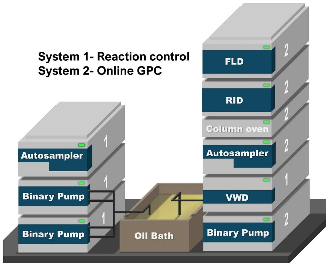
**Fig. 1** Schematic view of the flow reactor coupled to the online GPC. System 1 is a self-contained HPLC system consisting of two binary pumps, an autosampler and a UV detector. System 2 forms the online GPC, consisting of a binary HPLC pump, an autosampler, column oven fitted with variable wavelength UV (VWD), fluorescence (FLD) and differential refractive index (DRI) detectors.
