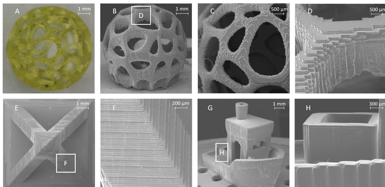
**Fig. 6** Show-prints of the formulation containing the trioxane triene and trithiol CHTT: (A) digital microscope image of hollow ball structure and corresponding SEM images: (B) full structure, (C) close-up, (D) bar. SEM images of hollow pyramid displaying (E) top view and (F) side bar detail. SEM image of benchy displayed (G) in full and (H) from the side at larger resolution.
