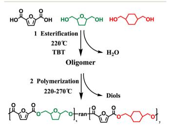
**Fig. 3** Schematic representation of the synthesis of poly(1,4-cyclohexyldimethylene-co-hydroxymethyl tetrahydrofuran 2,5-furandicarboxylate) (PCTF) from FDCA, BHMTHF and CHDM. Figure adapted and reproduced with permission from ref. 37. Copyright 2021 ACS Sustainable Chem. Eng.
