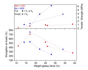
Fig. 10 Comparison of copolymers elongation (lower panel) and tensile strength (upper panel) versus glassy block (Red symbols represent CECs while blue ones BEBs; full symbols represent copolymers made with E1 or E2 as macroCTA, while empty symbols are for copolymers made by E3).
