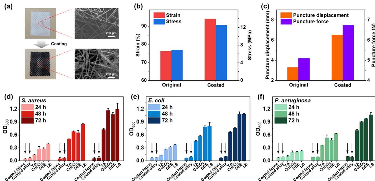
**Fig. 6** (a) SEM images of original and coated non-woven fabrics. (b) Strain and stress curves of original and coated non-woven fabrics. (c) Puncture force and displacement of original and non-coated woven fabrics. Antibacterial ability of the titanium alloy and non-woven fabric coated with Poly(TA-DES<sub>10</sub>-Cu<sub>8</sub>), TA, CuSO<sub>4</sub> and DES, respectively, against (d) *S. aureus*, (e) *E. coli*, and (f) *P. aeruginosa*.
