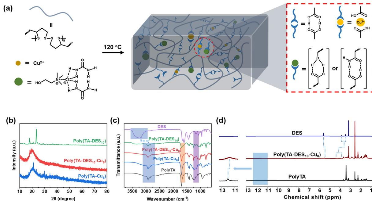
Fig. 1 (a) The schematic representation of Poly(TA-DES-Cu) preparation. (b) PXRD spectra of Poly(TA-DES<sub>10</sub>), Poly(TA-DES<sub>10</sub>-Cu<sub>8</sub>), and Poly(TA-Cu<sub>8</sub>). (c) ATR-FTIR spectra of DES, Poly(TA-DES<sub>10</sub>), Poly(TA-DES<sub>10</sub>-Cu<sub>8</sub>), Poly(TA-Cu<sub>8</sub>), and PolyTA. (d) <sup>1</sup>H NMR spectra of DES, Poly(TA-DES<sub>10</sub>-Cu<sub>8</sub>), and PolyTA (400 MHz, DMSO-*d*<sub>6</sub>, 298 K).
