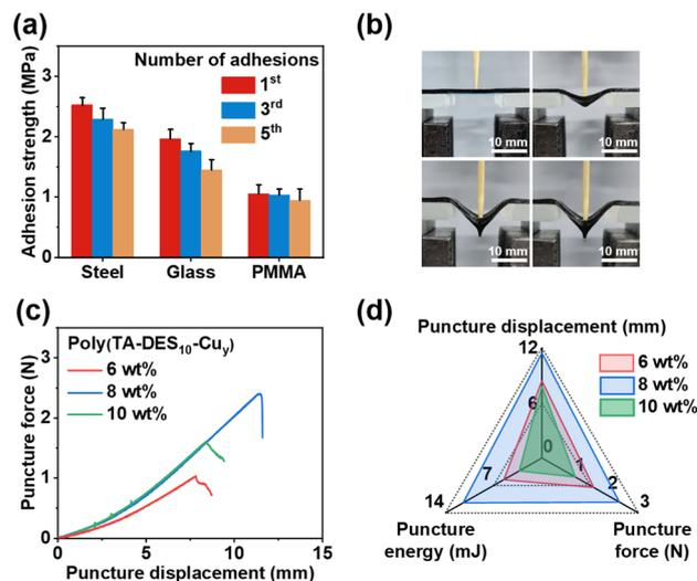
Fig. 5 (a) Continuous cyclic adhesion tests of Poly(TA-DES<sub>10</sub>-Cu<sub>8</sub>) on different substrates. (b) Photographs of Poly(TA-DES<sub>10</sub>-Cu<sub>8</sub>) during the puncture test. (c) Puncture force-displacement curves of Poly(TA-DES<sub>10</sub>-Cu<sub>8</sub>) with different weight ratios of Cu<sup>2+</sup> ( $y = 6, 8$  and  $10$ , respectively). (d) Puncture displacement, puncture force and puncture energy of Poly(TA-DES<sub>10</sub>-Cu<sub>8</sub>).
