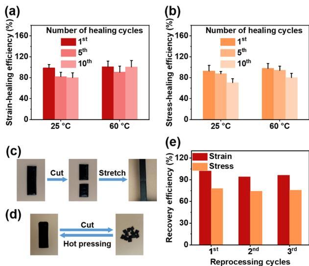
Fig. 4 Self-healing efficiency of Poly(TA-DES<sub>10</sub>-Cu<sub>8</sub>) at 25 and 60 °C: (a) strain, (b) stress, and (c) photographs of the self-healing of Poly(TA-DES<sub>10</sub>-Cu<sub>8</sub>) that was cut into two pieces. (d) Recycling of Poly(TA-DES<sub>10</sub>-Cu<sub>8</sub>) by hot pressing. (e) Recovery efficiency of Poly(TA-DES<sub>10</sub>-Cu<sub>8</sub>).
