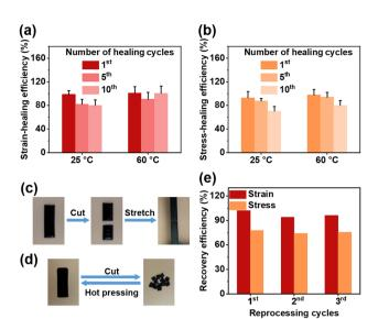
Fig. 4 Self-healing efficiency of  $Poly(TA-DES_{10}-Cu_8)$  at 25 and 60 °C: (a) strain, (b) stress, and (c) photographs of the self-healing of  $Poly(TA-DES_{10}-Cu_8)$  that was cut into two pieces. (d) Recycling of  $Poly(TA-DES_{10}-Cu_8)$  by hot pressing. (e) Recovery efficiency of  $Poly(TA-DES_{10}-Cu_8)$ .
