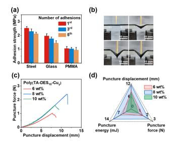
Fig. 5 (a) Continuous cyclic adhesion tests of  $Poly(TA-DES_{10}-Cu_8)$  on different substrates. (b) Photographs of  $Poly(TA-DES_{10}-Cu_8)$  during the puncture test. (c) Puncture force–displacement curves of  $Poly(TA-DES_{10}-Cu_y)$  with different weight ratios of  $Cu^{2+}$  (y=6, 8 and 10, respectively). (d) Puncture displacement, puncture force and puncture energy of  $Poly(TA-DES_{10}-Cu_y)$ .
