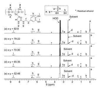
Fig. 2 <sup>1</sup>H NMR spectra in DMSO- $d_6$  of PDMS-PS-Ph(OH)<sub>2</sub> (x:y); x:y = (a) 9:1, (b) 8:2, (c) 7:3, (d) 6:4 and (e) 5:5. Chemical shifts are referenced to DMSO- $d_6$  ( $\delta$  2.5).
