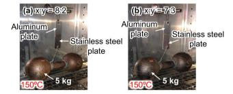
Fig. 7 Evaluation of adhesiveness at high temperatures (150 °C) between the aluminum and stainless-steel plates adhered using PDMS-PS-Ph(OH)<sub>2</sub> (x:y); x:y=(a) 8:2 and (b) 7:3.
