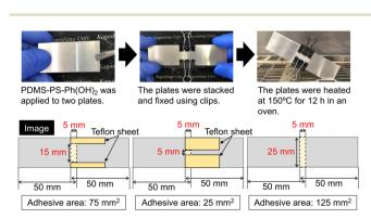
Fig. 3 Method of adhesion between the adherends (e.g., aluminum plates) using PDMS-PS-Ph(OH)<sub>2</sub> (x : y).
