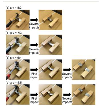
Fig. 5 Evaluation of adhesiveness under impact loads for the aluminum plates adhered using PDMS-PS-Ph(OH)<sub>2</sub> (x:y); x:y=(a) 8:2, (b) 7:3, (c) 6:4 and (d) 5:5.
