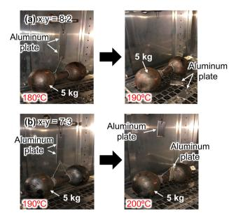
Fig. 6 Evaluation of adhesiveness at high temperatures for the aluminum plates adhered using PDMS-PS-Ph(OH)<sub>2</sub> (x:y); x:y = (a) 8:2 and (b) 7:3.
