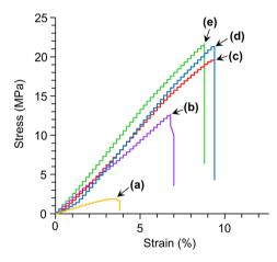
Fig. 4 Stress-strain curves obtained via the tensile shear tests of the aluminum plates adhered using PDMS-PS-Ph(OH)<sub>2</sub> (x:y); x:y=(a) 9:1, (b) 8:2, (c) 7:3, (d) 6:4 and (e) 5:5.
