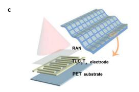
**Fig. 24** Reports of telluophene-based polymers in OPD applications. (a) Polymeric structures of PBTT and PBTB used in short-wave infrared (SWIR) OPDs. (b) Structure of RAN polymer used in the NIR  $Ti_3C_2T_x$ -RAN PD. (c) Schematic diagram of single  $Ti_3C_2T_x$ -RAN PD structure. Reproduced from ref. 119 with permission from John Wiley and Sons, copyright 2022.
