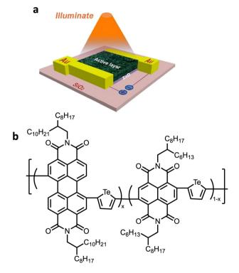
Fig. 23 Application of tellurophene-containing polymer in an OPD. (a) Device architecture for the photodetectors with SiO₂/ZnO/polymer/Au configuration. (b) Structure of random copolymers of PDI/NDI with tellurophene. Reproduced from ref. 116 with permission from American Chemical Society, copyright 2018.
