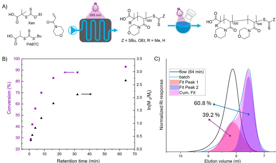
**Fig. 5** Flow chemistry experiment using an 8 mL coil within a photo reactor to produce PNAM500 first block to be chain extended with a second block of NAM in batch reaction. (A) Schematic overview over the reaction. (B) Conversion as a function of time within the coil. (C) SEC traces of initial PNAM and after chain extension including peak deconvolution (deconvolution data presented in Fig. S8†).
