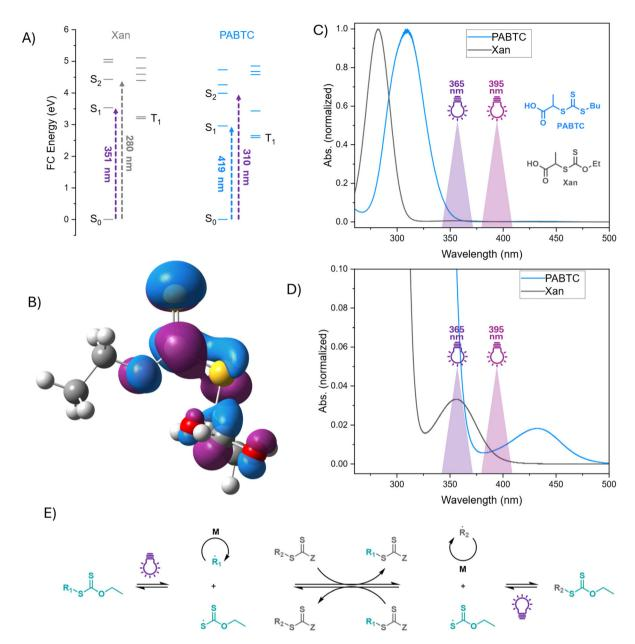
Fig. 1 (A) Energy levels of electronic transitions in Xan and PABTC from DFT calculations. (B) Illustration of the NTO of the S2 state for Xan. (C & D) UV Vis spectra of both CTAs in DMSO (c = 0.156 mM (C), c = 1.25 mM (D)) with indications of the light wavelengths used in this work. (E) Schematic representation of the XPI-RAFT concept.
