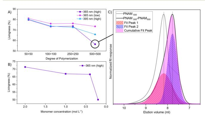
Fig. 4 Livingness of pseudo diblock copolymers based on XPI-RAFT polymerization at different reaction conditions. (A) Livingness as extrapolated from deconvolution of SEC traces for polymerization reactions at different DP values and irradiation conditions. (B) Livingness at constant DP (500 + 500) as a function of monomer (and CTA) concentration. (C) Exemplary deconvolution of SEC traces where peak maxima are based on the maxima of first and second block (performed in Origin software).
