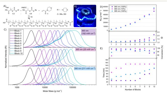
Fig. 2 Synthesis of pseudo block copolymers using NAM, Xan and PABTC at different irradiation conditions. (A) Schematic overview of the synthesis and target structure. (B) PhotoCube from ThalesNano used to conduct photopolymerizations. (C) SEC traces calibrated (THF, PS calibration) showing chain extension for 10 blocks. (D) Evolution of  $M_n$  and D upon chain extension, (E) reaction time necessary to reach a conversion of >90% for each block and irradiation condition.
