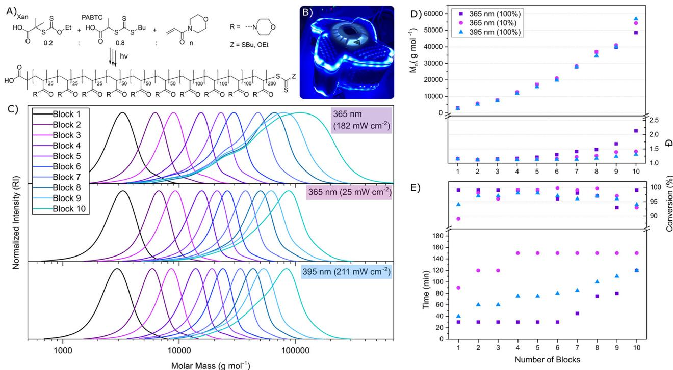
**Fig. 2** Synthesis of pseudo block copolymers using NAM, Xan and PABTC at different irradiation conditions. (A) Schematic overview of the synthesis and target structure. (B) PhotoCube from ThalesNano used to conduct photopolymerizations. (C) SEC traces calibrated (THF, PS calibration) showing chain extension for 10 blocks. (D) Evolution of  $M_n$  and  $\bar{D}$  upon chain extension, (E) reaction time necessary to reach a conversion of >90% for each block and irradiation condition.
