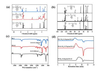
Fig. 1 (a) <sup>1</sup>H NMR analysis in d6-DMSO, (b) <sup>13</sup>C NMR analysis in d6-DMSO, (c) FT-IR spectrum and (d) GPC analysis of P0, P0-0.6 & P0-2.
