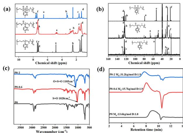
**Fig. 1** (a) <sup>1</sup>H NMR analysis in d<sub>6</sub>-DMSO, (b) <sup>13</sup>C NMR analysis in d<sub>6</sub>-DMSO, (c) FT-IR spectrum and (d) GPC analysis of P0, P0-0.6 & P0-2.
