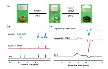
Fig. 5 (a) Photographs showing the treatment of P0-2 in DMSO and DMSO-DBU: (b) <sup>1</sup>H NMR and (c) GPC analyses of P0-2 before and after the degradation study.
