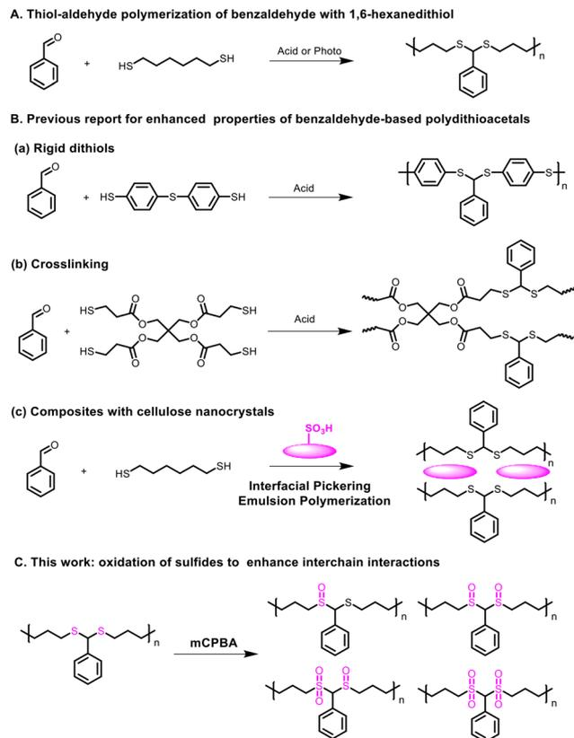
**Scheme 1** (A) Polydithioacetals from the polycondensation between benzaldehyde and 1,6-hexanedithiol, (B) strategies to enhance the mechanical properties of benzaldehyde-based polydithioacetals, and (C) oxidation of sulfides to enhance interchain interactions.
