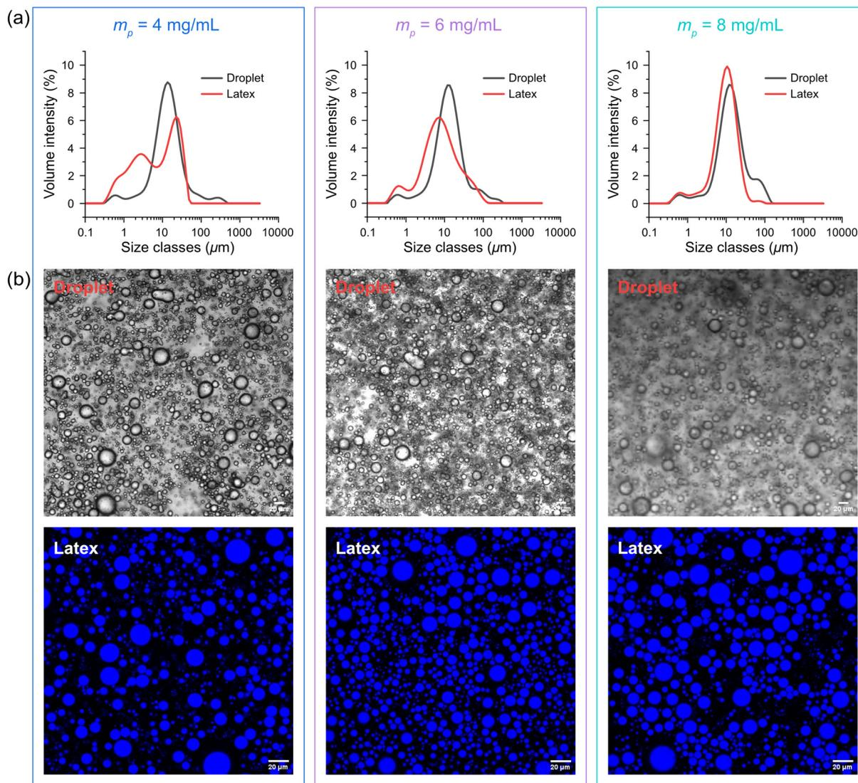
**Fig. 3** (a) Size distributions and (b) confocal microscopy images of the HCC/siloxane amine emulsion droplets and WNIPU latexes with CNC concentrations ( $m_p$ ) of 4, 6, and  $8 \text{ mg mL}^{-1}$ . Scale bar:  $20 \text{ }\mu\text{m}$ .
