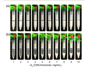
Fig. 1 HCC/siloxane amine/aqueous CNC emulsion stability with increasing CNC concentration in the aqueous phase. Photographs of (a) the emulsions freshly prepared using Ultra-Turrax, and (b) the emulsions stored for 3 h after emulsification.
