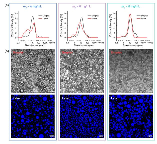
Fig. 3 (a) Size distributions and (b) confocal microscopy images of the HCC/siloxane amine emulsion droplets and WNIPU latexes with CNC concentrations ( $m_p$ ) of 4, 6, and 8 mg mL<sup>-1</sup>. Scale bar: 20  $\mu$ m.
