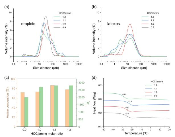
Fig. 6 Effect of the HCC/amine ratio on (a) droplet size distribution, (b) latex size distribution, and (c) amine conversion determined by  $^1$ H NMR and  $\overline{M}_n$  determined using polystyrene standards on SEC, and (d) DSC thermograms from the second heating ramp of WNIPU latexes stabilized with a CNC concentration at an  $m_p$  of 8 mg mL<sup>-1</sup>.
