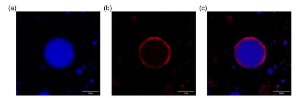
Fig. 4 Confocal laser scanning microscopy (CLSM) images of the WNIPU latex stabilized with CNC-RB at an  $m_p$  of 8 mg mL<sup>-1</sup>. (a) Fluorescence detected under 405 nm excitation (WNIPU), (b) fluorescence detected under 561 nm excitation (CNC-RB), and (c) merged image of both channels. Scale bar: 10 µm.
