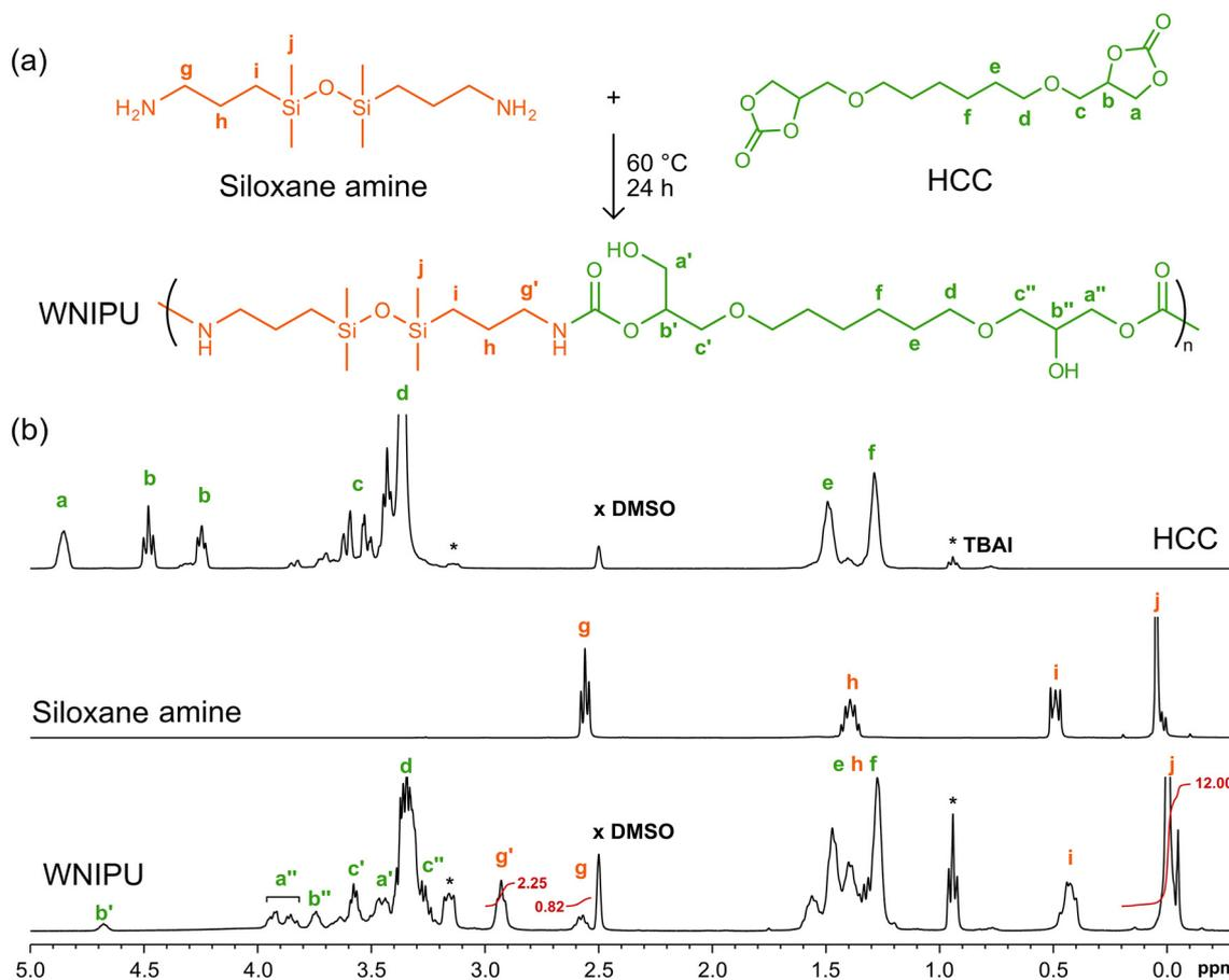
Fig. 5 (a) Reaction scheme between siloxane amine and HCC. (b) <sup>1</sup>H NMR spectra of starting monomers HCC, siloxane amine and the dried WNIPU latex with an HCC/amine ratio of 1.0 in a mixture of CDCl<sub>3</sub> and DMSO-*d*<sub>6</sub>.
