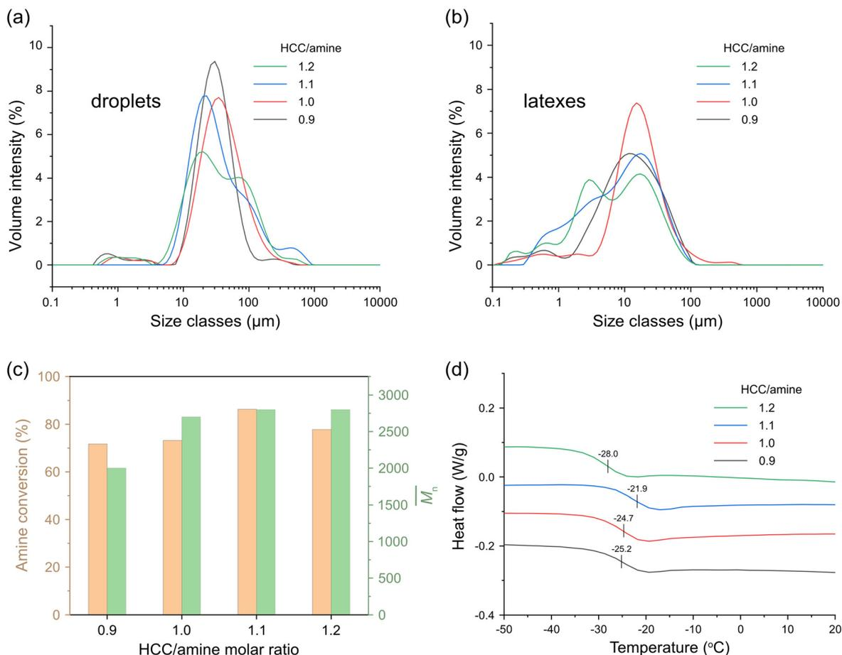
**Fig. 6** Effect of the HCC/amine ratio on (a) droplet size distribution, (b) latex size distribution, and (c) amine conversion determined by  $^1\text{H}$  NMR and  $M_n$  determined using polystyrene standards on SEC, and (d) DSC thermograms from the second heating ramp of WNIPU latexes stabilized with a CNC concentration at an  $m_p$  of  $8 \text{ mg mL}^{-1}$ .
