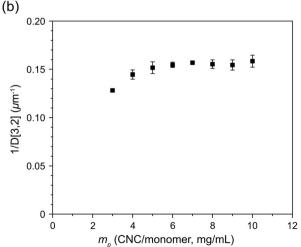
Fig. 2 (a) Size distribution and (b) the inverse D[3,2] average diameters of the HCC/siloxane amine emulsion droplets as a function of CNC concentration ( $m_p$  of 3 to 10 mg ml<sup>-1</sup>).
