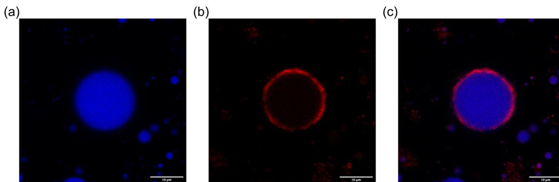
Fig. 4 Confocal laser scanning microscopy (CLSM) images of the WNIPU latex stabilized with CNC-RB at an  $m_p$  of  $8 \text{ mg mL}^{-1}$ . (a) Fluorescence detected under 405 nm excitation (WNIPU), (b) fluorescence detected under 561 nm excitation (CNC-RB), and (c) merged image of both channels. Scale bar:  $10 \text{ }\mu\text{m}$ .
