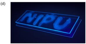
Fig. 7 Photographs and fluorescence spectra of the aqueous WNIPU latex suspensions with varying solid contents. (a) Photographs taken under nature light, (b) photographs taken under UV irradiation ( $\lambda=365$  nm), and (c) excitation and emission spectra recorded with aqueous suspensions. (d) Photograph of the letters "NIPU" written on a glass slide using the aqueous WNIPU latex suspension as ink, taken under 365 nm UV light (letters were written on the top glass slide).
