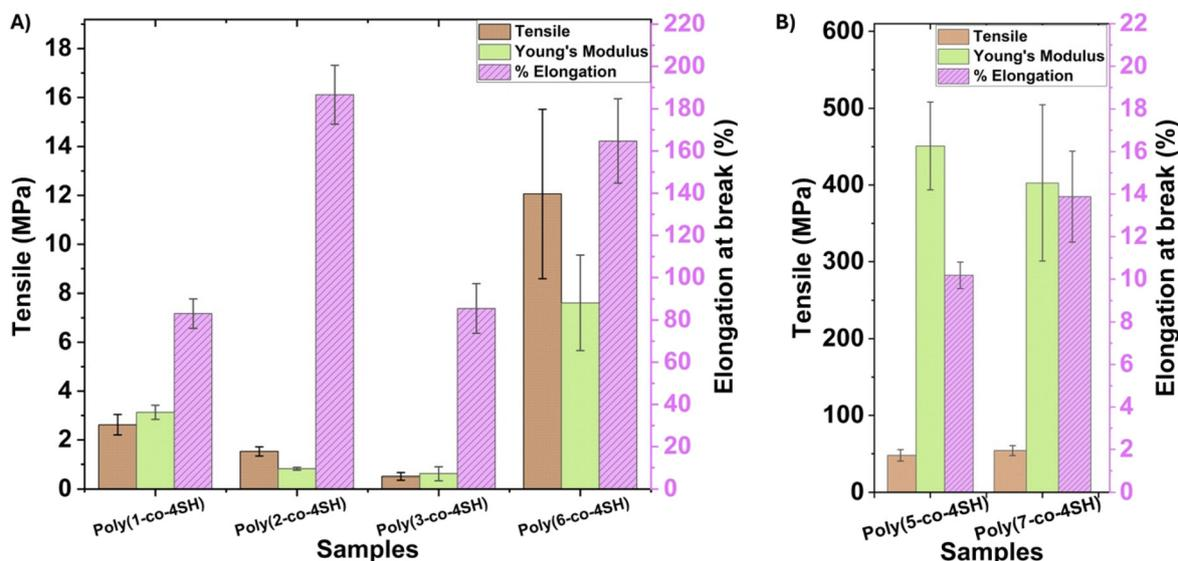
**Fig. 3** Mechanical analysis of LGO-based thiol-ene networks: (A) soft polymers and (B) firm polymers (error bars indicate the standard deviation, left Y-axis represents tensile strength and Young's modulus and right Y-axis represents % elongation at break).
