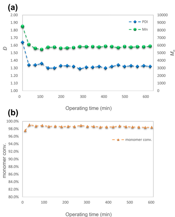
Fig. 5 Droplet flow of GTP for a 600 min operating time. [MMA]_0/[MTS]_0/[P_4-t-Bu] = 50/1/0.001 , (MMA + MTS)/(PEGMEA) = 30/70 in weight, flow length: 9.0 m with i.d. of 3.0 mm, (a) \bar{D} values and M_n , and (b) monomer conversion with different sampling times.
