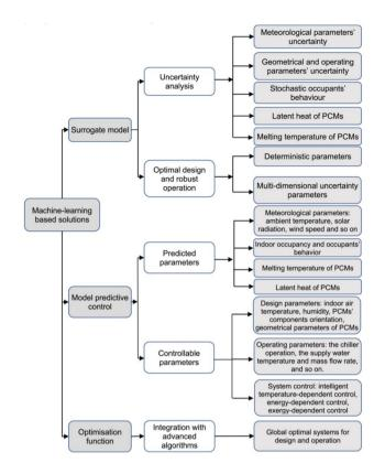
Fig. 9 Application of the machine learning method in novel PCMs cooling systems.  $^{110}$
