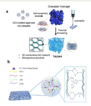
**Fig. 8** (a) Schematic illustration of the fabrication of a thermally annealed graphene-connected agarose hydrogel. <sup>87</sup> GO-coated agarose microbeads were self-assembled to form GHs, and after thermal annealing, TAGAH was formed. (b) Illustration of the synthesis of self-healing hydrogel composites loaded with graphene nanoplatelets; <sup>67</sup> dynamic cross-linking exists between the PAA chains and Fe<sup>3+</sup>.
