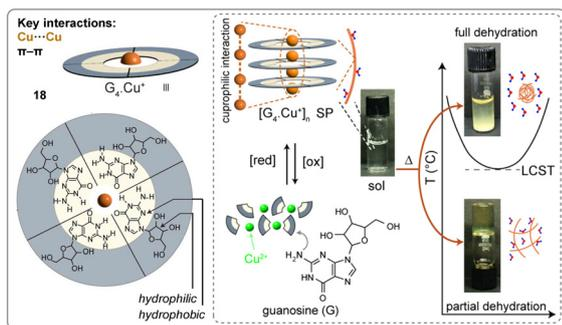
**Fig. 15** Structure of Cu(I) guanosine (G)-quadruplex **18** and inlay of its supramolecular polymer showing a thermoresponsive LCST transition and redox responsive reversible depolymerization. Reproduced from ref. 22 with permission from Wiley, copyright 2025.
