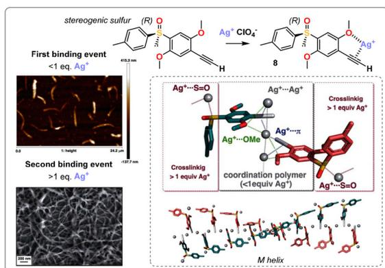
**Fig. 7** Structure of chiral phenylacetylene monomer **8** with AFM height image of **8** (1.0/0.6 ligand/Ag<sup>+</sup> molar ratio), SEM image of **8** (1.0/4.0 ligand/Ag<sup>+</sup> molar ratio) and inlay of Ag(I) complex **8** as well as the aggregation model for **8** showing the involved interactions and *M* chiral helix. Reproduced from ref. 46 with permission from Wiley, copyright 2024.
