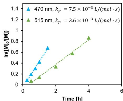
Fig. 3 Polymerisation kinetics initiated under  $\lambda_{\max} = 470$  and 515 nm,  $1.6$  mW cm<sup>-2</sup> in DMSO at a monomer concentration of 50 vol%,  $[M]_0/[I] = 100$ , 22 °C.
