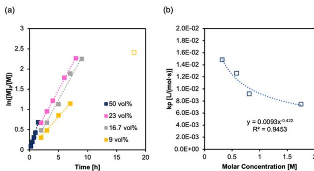
**Fig. 4** (a) Polymerisation kinetics at different monomer concentrations (50, 23, 17, and 9 vol%) in DMSO. Reaction kinetics at 50% v/v is polymer 1 reported in Fig. 3 and Table 1. Initiated under  $\lambda_{\max} = 470$  nm, 1.6 mW cm<sup>-2</sup> in DMSO,  $[M]_0/[I] = 100$ , 22 °C. The 18 h datapoint at 9% v/v is off trend and is excluded as an outlier, probably caused by the loss of active chain-ends. (b) Monomer concentration plotted against  $k_p$ .
