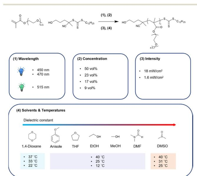
**Fig. 1** P(PEGMA) synthesis scheme through the PI-RAFT approach and overview of this study. The synthesis in 1,4-dioxane and DMSO cannot be conducted at 12 °C because of the high melting point of solvents.
