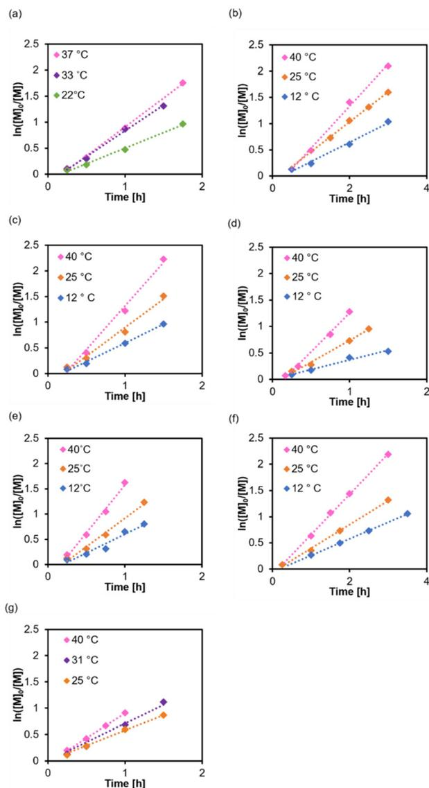
**Fig. 5** Polymerisation kinetics at different temperatures and in various solvents: (a) 1,4-dioxane, (b) anisole, (c) THF, (d) EtOH, (e) MeOH, (f) DMF, and (g) DMSO. Initiated under  $\lambda_{\max} = 450 \text{ nm}$ ,  $18 \text{ mW cm}^{-2}$ ,  $[M]_0/[I] = 100$ ,  $[M]_0 = 50 \text{ vol\%}$ .
