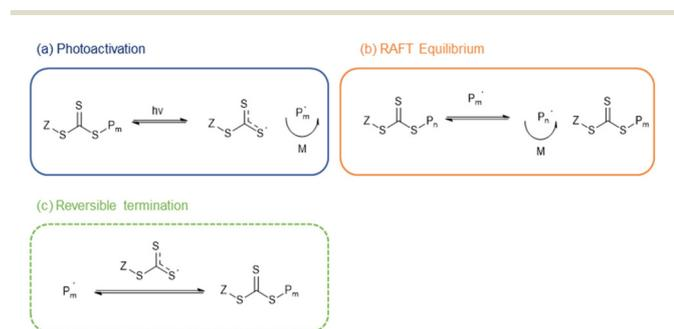
**Scheme 1** General mechanism of PI-RAFT polymerisation. The S–C bond is photolysed to generate a free radical (a, photoactivation). The propagating radical can either chain transfer the active centre (b, RAFT equilibrium) or combine with a photoiniferter radical to terminate reversibly (c, reversible termination).
