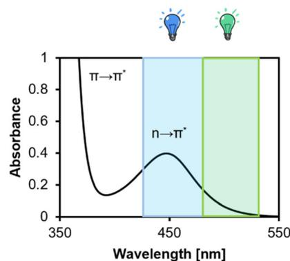
Fig. 2 Absorbance of CTA in DMSO, 5 mg mL<sup>-1</sup>.  $\pi \rightarrow \pi^*$  and  $n \rightarrow \pi^*$  transition as annotated in the spectrum. Shaded areas indicate the overlap of the excitation mechanism with wavelengths of light used in this study.
