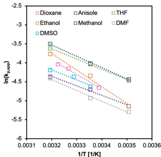
**Fig. 6** Arrhenius plot for PI-RAFT synthesis of PPEGMA in various solvents. Initiated under  $\lambda_{\max} = 450 \text{ nm}$ ,  $18 \text{ mW cm}^{-2}$ ,  $[M]_0/[I] = 100$ , 50 vol%.
