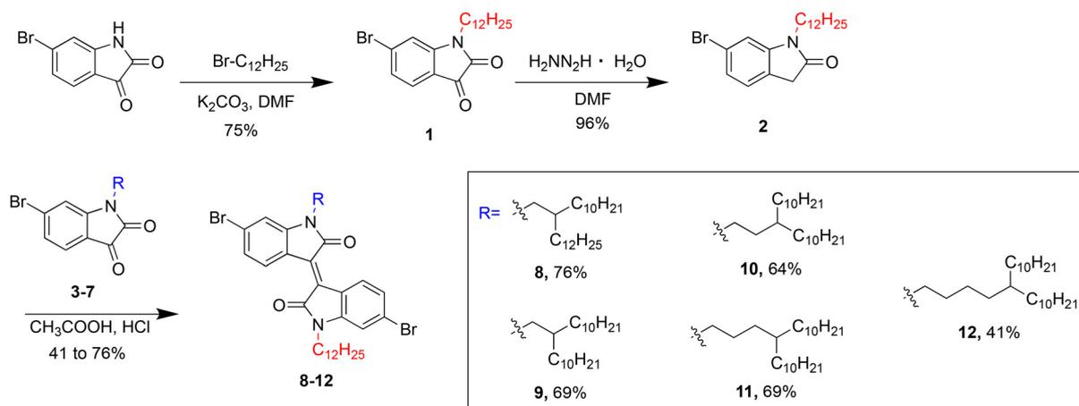
Scheme 1 Synthetic pathway to asymmetric isoindigo **ii**(C<sub>*n*</sub>C<sub>*x*</sub>C<sub>*y*</sub>)(C<sub>12</sub>) monomers, compounds **8** to **12**.
