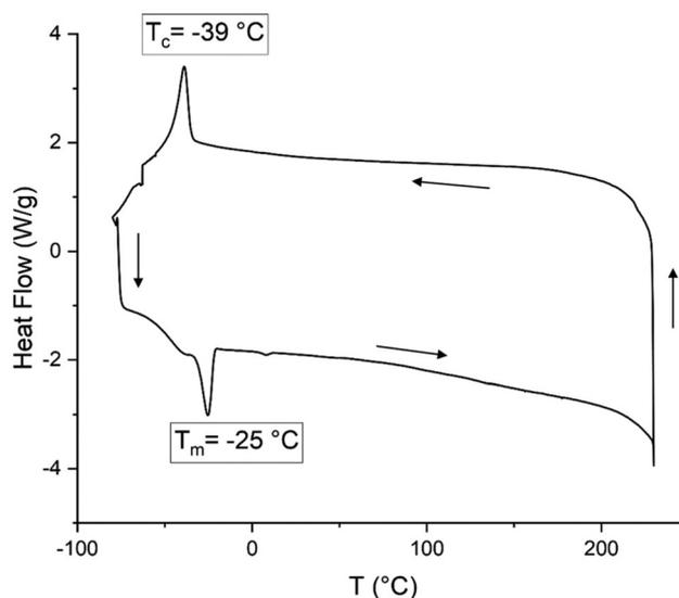
**Fig. 2** DSC analysis of PLC<sup>S</sup>, note that the data refer to the second heating/cooling.
