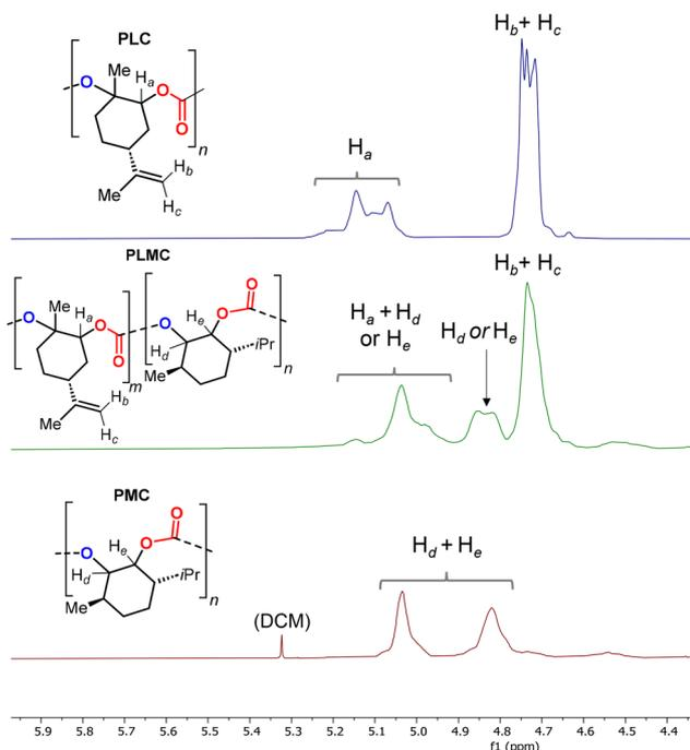
**Fig. 1**  $^1\text{H NMR}$  spectral comparison between **PLC**, **PMC** and the **PLMC** from entry 13 in Table 1. A selected zoom of the region where the methine and olefinic H are resonating is shown. For more detailed peak assignments, see the ESI, Fig. S53.†
