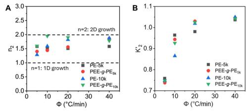
Fig. 10 (A) Avrami exponent and (B) Jeziorny-modified Avrami constant for non-isothermal crystallization of PE-5k, PEE-g-PE<sub>5k</sub>, PE-10k, and PEE-g-PE<sub>10k</sub>.
