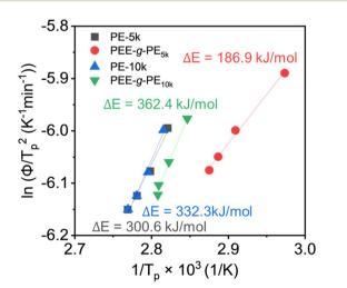
Fig. 11 Plots of  $\ln\left(\frac{\phi}{T_{\rm P}^2}\right)$  versus  $\frac{1}{T_{\rm P}}$  for PE-5k, PEE-g-PE<sub>5k</sub>, PE-10k, and PEE-g-PE<sub>10k</sub>.
