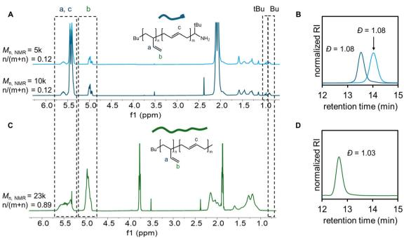
Fig. 2 (A) <sup>1</sup>H NMR spectra of 1,4-PB-NH<sub>2</sub> graft, (B) GPC result of 1,4-PB-NH<sub>2</sub> graft, (C) <sup>1</sup>H NMR spectrum of 1,2-PB backbone, and (D) GPC result of <sup>1</sup>H NMR of 1.2-PB backbone.
