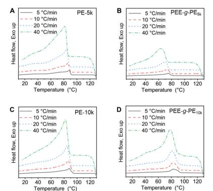
Fig. 8 DSC curves during non-isothermal crystallization at different cooling rates for (A) PE-5k, (B) PEE-g-PE<sub>5k</sub>, (C) PE-10k, and (D) PEE-g-PE<sub>10k</sub>.
