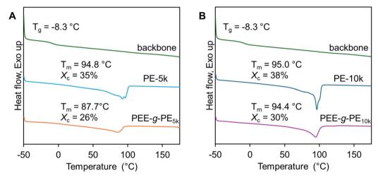
Fig. 7 DSC curves of (A) PEE-g-PE<sub>10k</sub>, hydrogenated 1,4-PB-NH<sub>2</sub> (graft-5k) and hydrogenated 1,2-PB-COOH (backbone), and (B) PEE-g-PE<sub>5k</sub>, hydrogenated 1,4-PB-NH<sub>2</sub> (graft-10k) and hydrogenated 1,2-PB-COOH (backbone), the crystallinity of PEE-q-PE was normalized by the mass ratio of PE over the total mass of the graft polymer.
