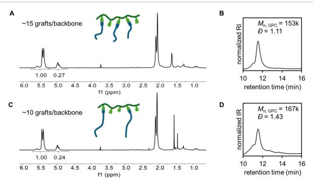
Fig. 5 (A) <sup>1</sup>H NMR of the isolated PBgp-5k, (B) GPC trace of the isolated PBgp-5k, (C) <sup>1</sup>H NMR of the isolated PBgp-10k, and (D) GPC trace of the isolated PBgp-10k.
