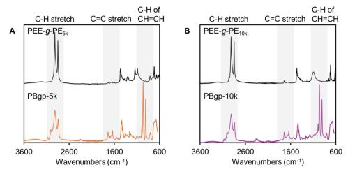
Fig. 6 FTIR of (A) PBgp-5k and the hydrogenated polymer PEE-g-PE<sub>5k</sub>, and (B) PBgp-10k and the hydrogenated polymer PEE-g-PE<sub>10k</sub>
