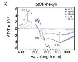
Fig. 3 Femtosecond time-resolved transient absorption data of (a) caro-PPV and (b) p(CP-hexyl) polymers prepared in chlorobenzene solution. Both caro-PPV and p(CP-hexyl) were pumped at 460 nm, with temporal resolution <200 fs and a laser power of  $400 \mu W$ .
