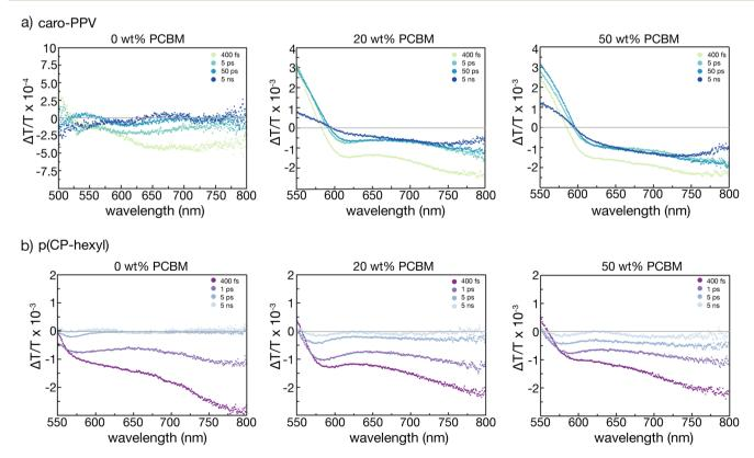
Fig. 4 Femtosecond time-resolved transient absorption graphs represented in terms of  $\Delta T/T$  of PCBM doped films (0, 20, 50 wt%) of (a) caro-PPV and (b) p(CP-hexyl) polymers. Both caro-PPV and p(CP-hexyl) were pumped at 460 nm, with temporal resolution <200 fs and a laser power of 400  $\mu$ W.
