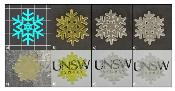
Fig. 6 3D Printing of complex snowflake structures. (a) Digital model. (b–e) Photographs of 3D-printed snowflakes using resins formulated with (b)  $PCL_{3k}$ –BTPA, (c)  $PCL_{3k}$ -acrylate, (d)  $PCL_{3k}$ -methacrylate, and (e)  $PCL_{3k}$ -OH (control). [AA]/[PEGDA] = 9/1 (molar ratio); PCL-R = 19 wt%; toluene = 10 wt%; and TPO = 1 wt%. Layer thickness: 50 µm. Cure times: 30 s ( $PCL_{3k}$ -BTPA and  $PCL_{3k}$ -OH) and 20 s (PCL-acrylate and  $PCL_{3k}$ -methacrylate).
