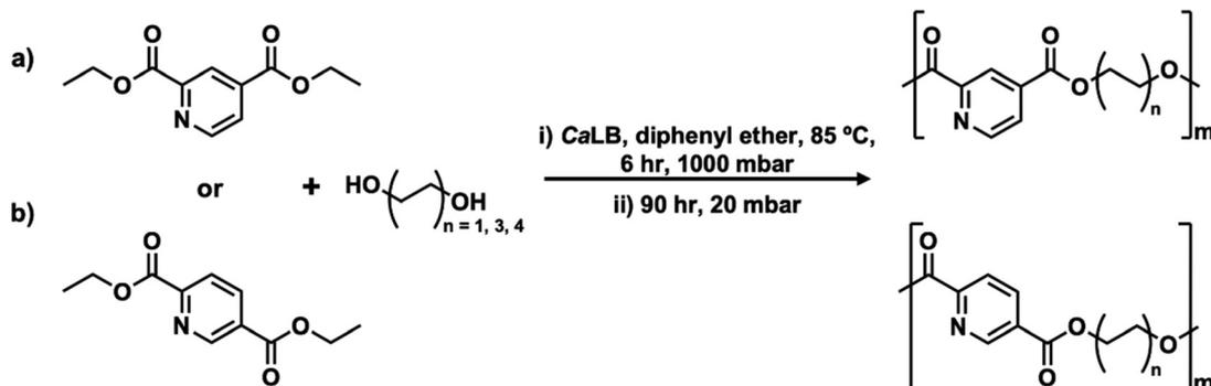
**Scheme 16** Polycondensation of 2,4 (a) and 2,5-dipyridinecarboxylic acid (b) with differing chain length alkyldiols.<sup>202</sup>
