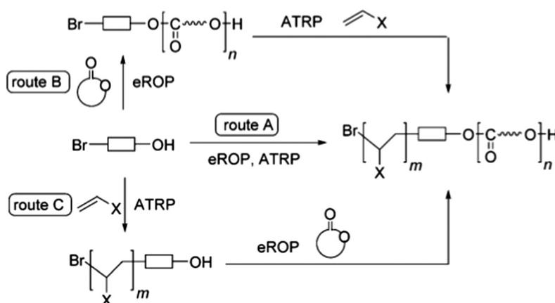
**Scheme 11** Combined enzymatic ATRP/eROP to produce general diblock copolyester through three routes. Route (A) Simultaneous eROP/ATRP. Route (B) eROP with bifunctional initiator, followed by ATRP. Route (C) ATRP with bifunctional initiator, followed by eROP. Reproduced from ref. 21, with permission from the American Chemical Society, copyright 2016.
