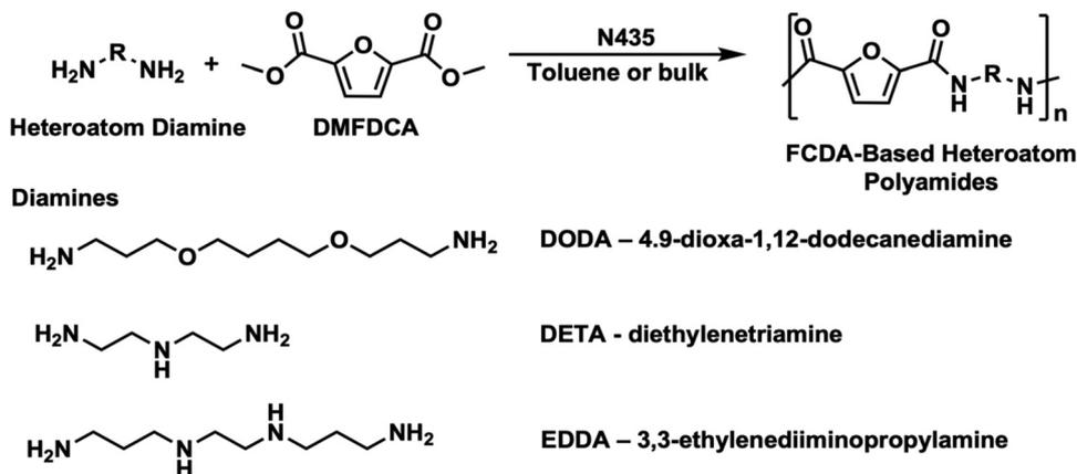
**Scheme 19** FDCA-heteroatom containing polyamides synthesised using N435.<sup>219</sup>
