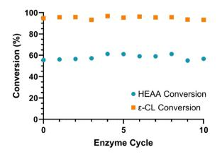
Fig. 11 Mean percentage conversion of CL and HEAA after 5 h of reaction (65 °C, 2-MeTHF, 10 wt% N435,  $\epsilon$ -CL concentration of 0.143 g mL $^{-1}$ ) whilst recycling the N435 beads (experiments run in triplicate). Adapted from ref. 121, with permission from the Royal Society of Chemistry, copyright 2022.
