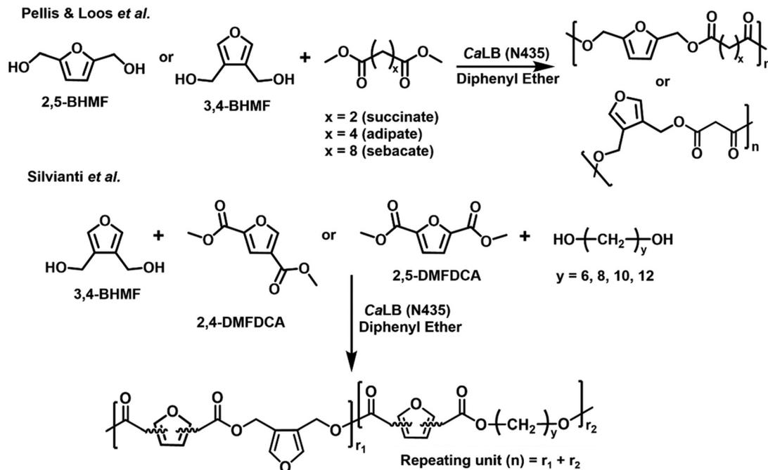
**Scheme 15** Enzymatic polycondensation using either furanic diols or methyl diesters, from the work of Pellis *et al.*<sup>190</sup> and Silvianti *et al.*<sup>195</sup>
