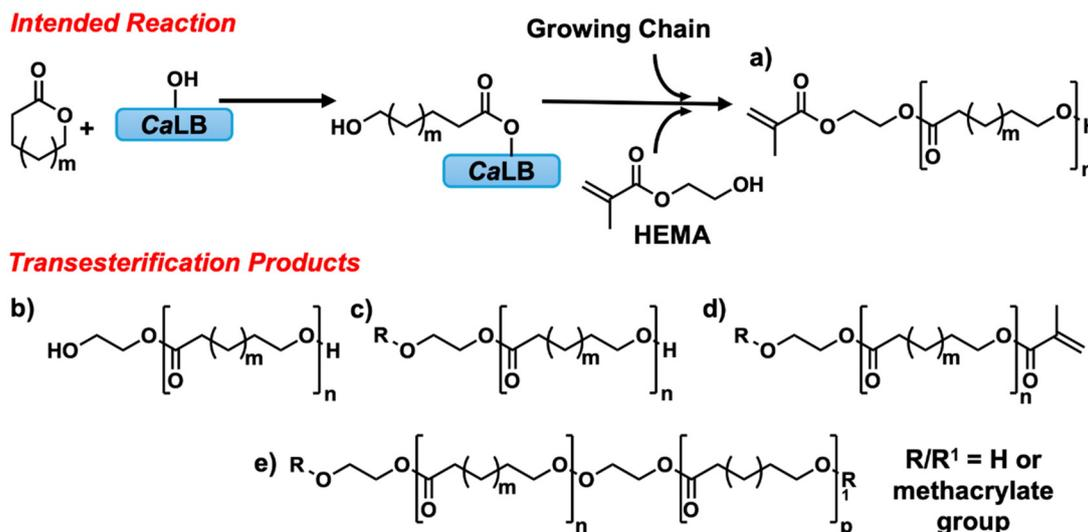
**Scheme 10** CaLB catalysed ROP of PDL ( $m = 11$ ) and CL ( $m = 2$ ), initiated by HEMA (product a). Transesterification products (b, c and d) formed from methacrylate transfer from HEMA end group of polymer to hydroxy end group, and (e) polyester transfer to the hydroxyl group of the residual 1–2-ethanediol end group.
