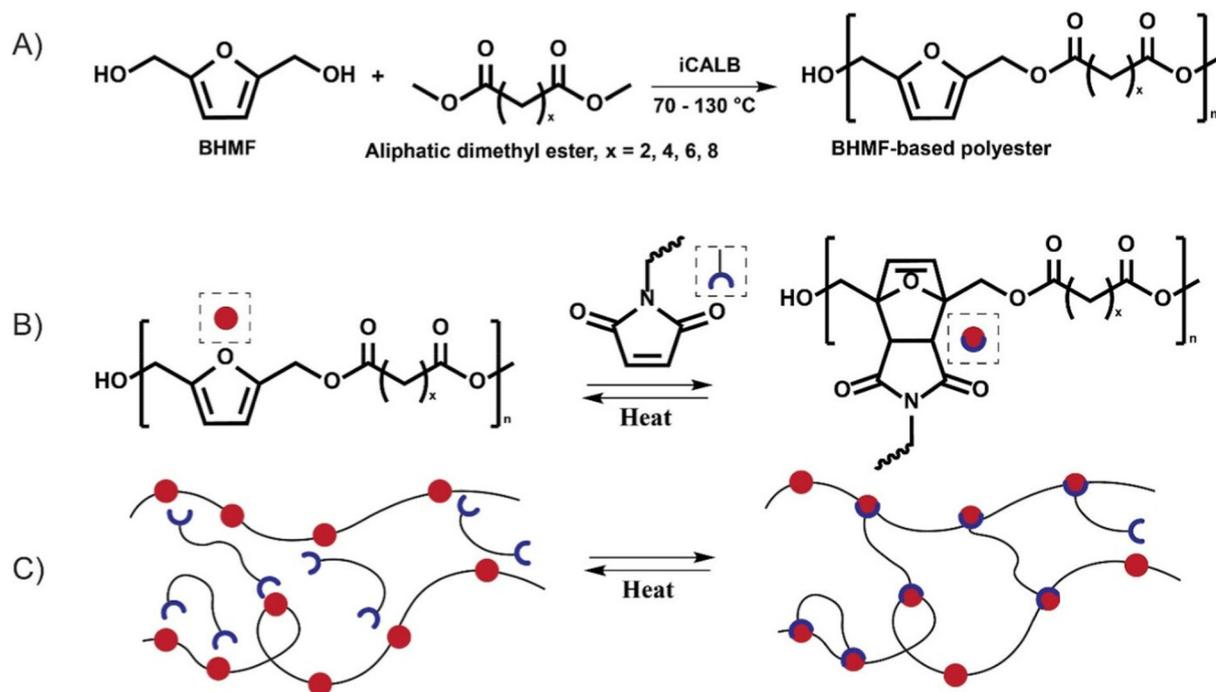
**Fig. 10** (A) Enzymatic polymerisation of 1,5-BHMF with a range of aliphatic dimethyl esters in bulk. (B) Reaction (via solvent casting) of the BHMF-based polyesters with a maleimide group. (C) Schematic overview of the thermoreversible Diels–Alder cross-linking of furanic polyester units with the bismaleimide units. Reproduced from ref. 197, with permission from the American Chemical Society, copyright 2025.
