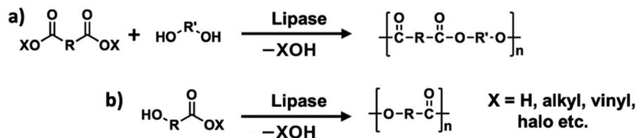
**Scheme 13** Lipase synthesised polyesters formed by (a) polycondensation of dicarboxylic acids or their esters with a diol (AA-BB polycondensation) and (b) self-polycondensation with oxyacids or their esters (AB polycondensation).
