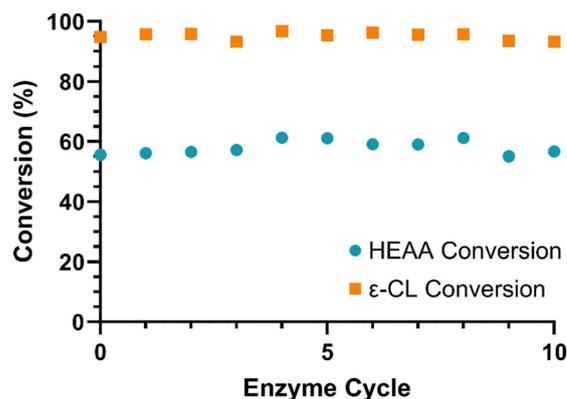
**Fig. 11** Mean percentage conversion of CL and HEAA after 5 h of reaction (65 °C, 2-MeTHF, 10 wt% N435,  $\epsilon$ -CL concentration of 0.143 g mL<sup>-1</sup>) whilst recycling the N435 beads (experiments run in triplicate). Adapted from ref. 121, with permission from the Royal Society of Chemistry, copyright 2022.
