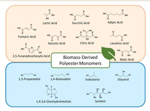
Fig. 7 Biomass derived diacid/diol/polyol monomers for use in step-growth enzymatic esterification reactions, note the undefined stereochemistry of 1,4:3,6-dianhydrohexitols represents 3 different possible stereoisomers.
