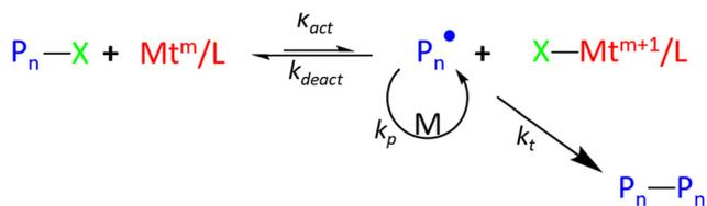
**Scheme 7** ATRP Mechanism (note charges and counterions are omitted for simplicity).  $P_n$ ,  $X$ ,  $Mt$ ,  $m$ ,  $L$  and  $M$  represent the alkyl chain, halide, transition metal, oxidation state and monomer respectively., adapted from ref. 57, with permission from the American Chemical Society, copyright 2012.
