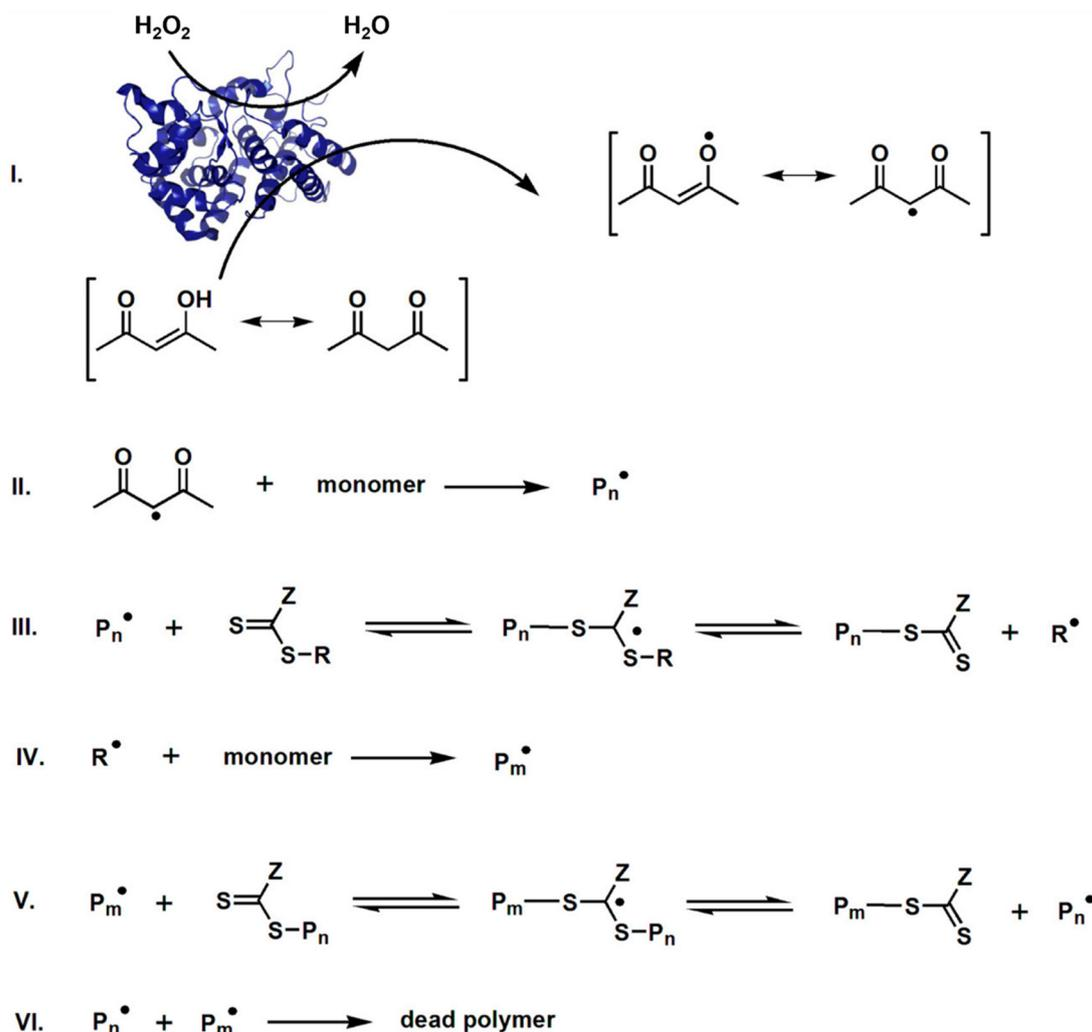
Fig. 4 Proposed mechanism of HRP initiated RAFT polymerisation. P<sub>n</sub> & P<sub>m</sub> represent propagating polymer chains whilst R and Z are substituents on the CTA. Reproduced from ref. 94, with permission from American Chemical Society, copyright 2015.
