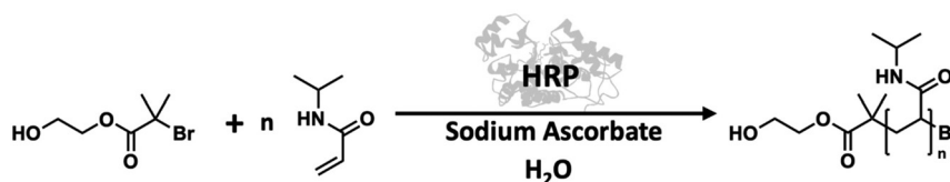
Scheme 8 HRP initiated ARGET ATRP of N -isopropyl acrylamide.
