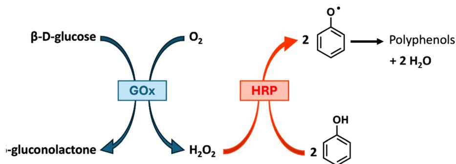
Scheme 3 GOx/HRP mediated radical initiation/polymerisation of phenol.
