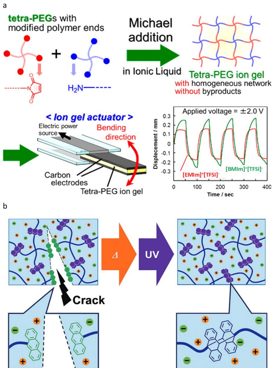
**Fig. 5** Schematics of ionogels with HNs. (a) Preparation of HN ionogels through Aza-Michael addition reaction and schematic configuration of polymer actuator. Adapted with permission.<sup>86</sup> Copyright 2017 American Chemical Society. (b) A conceptual illustration of photohealing of the 4-arm PEG ionogel. Adapted with permission.<sup>89</sup> Copyright 2018 The Royal Society of Chemistry.
