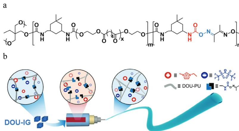
**Fig. 11** Structure and preparation of Di-Canogel fibers. (a) The chemical structure of Di-Canogels. (b) The manufacture process of Di-Canogel fibers. Adapted with permission.<sup>149</sup> Copyright 2024 Wiley.
