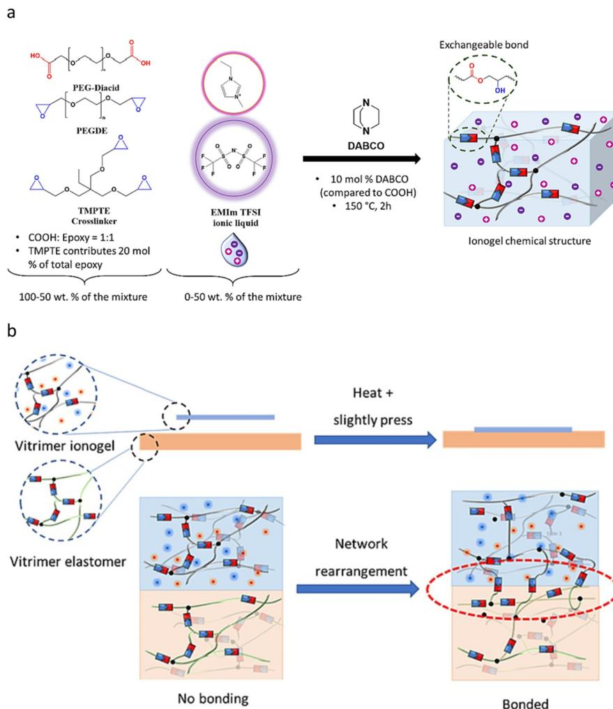
**Fig. 14** Structure and welding process of Ai-Canogels. (a) Composition and synthesis route of Ai-Canogels. (b) The manufacture process of multi layer materials by interface welding. Adapted with permission.<sup>177</sup> Copyright 2023 Elsevier.
