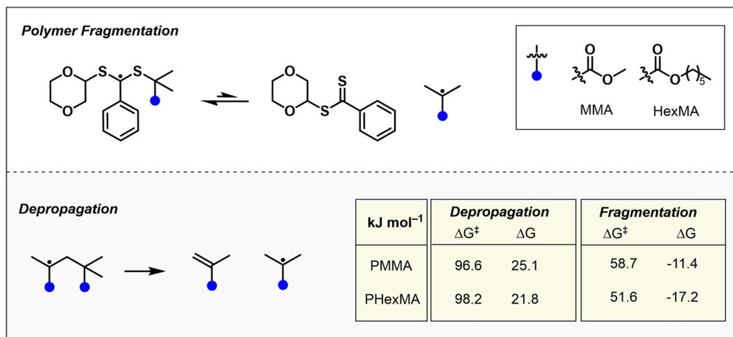
Fig. 3 Gibbs free energy barriers and reaction energies ( $\text{kJ mol}^{-1}$ ,  $120^\circ\text{C}$ ) as calculated at the wB97X-D/aug-cc-pVTZ//M062X/6-31G(d) level of theory using SMD to model the 1,4-dioxane solvent environment.
