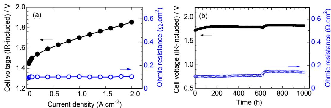
Fig. 11 (a) IR-included  $I$ - $V$  curve of the QBPh-Pip (IEC = 1.9 mequiv.  $g^{-1}$ ) cell at 80 °C with a 1 M KOH aqueous solution. (b) The durability of the QBPh-Pip (IEC = 1.9 mequiv.  $g^{-1}$ ) cell at 80 °C with a 1 M KOH aqueous solution.
