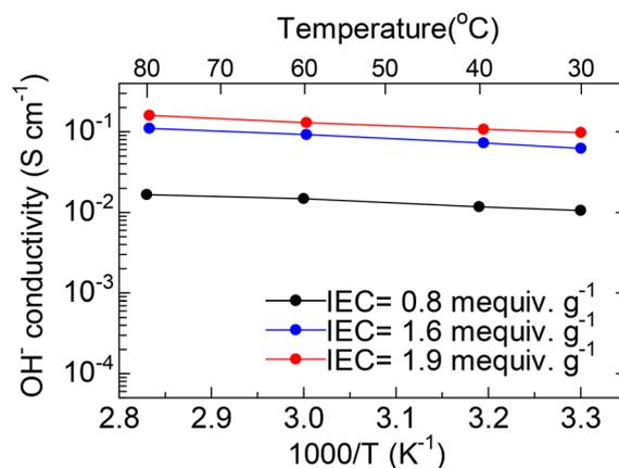
Fig. 6 Temperature dependence of  $\text{OH}^-$  conductivity of the different QBPh-Pip membranes.
