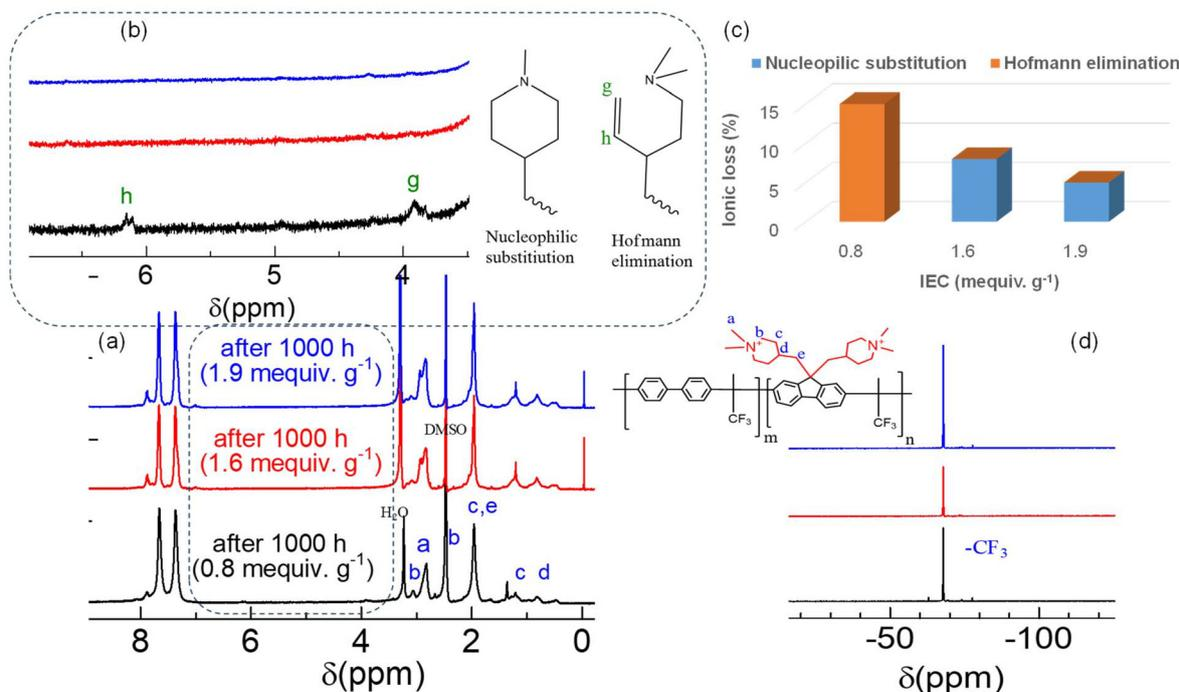
Fig. 8 (a) Post-test  $^1\text{H}$  NMR spectra of QBPh-Pip membranes after 1000 h in 8 M KOH at 80 °C, (b) magnified  $^1\text{H}$  NMR spectra, (c) IEC loss (%) estimated from the NMR integrals as a function of IEC, and (d)  $^{19}\text{F}$  NMR spectra of the post-test QBPh-Pip.
