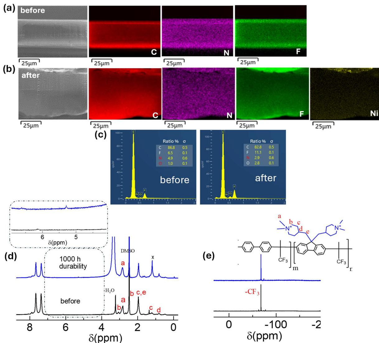
Fig. 12 SEM-EDS images of (a) initial and (b) postdurability QBPh-Pip (IEC = 1.9 mequiv.  $\text{g}^{-1}$ ) membranes. (c) Elemental analysis (EDS). (d)  $^1\text{H}$  and (e)  $^{19}\text{F}$  NMR spectra of QBPh-Pip (IEC = 1.9 mequiv.  $\text{g}^{-1}$ ) before and after 1000 h of durability testing.
