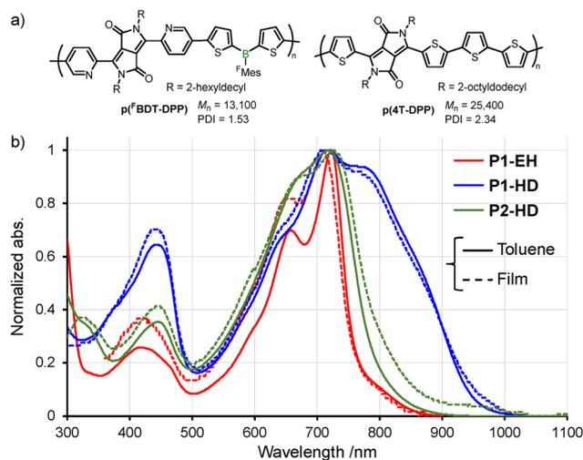
**Fig. 2** Chemical structures of previously reported DPP polymers (a) and UV-vis absorption spectra of DTSB/DTSO<sub>2</sub>B-containing polymers in toluene and as film (b).
