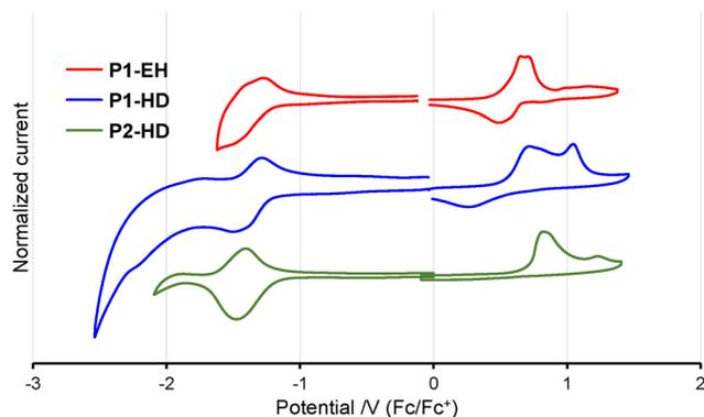
Fig. 4 Cyclic voltammograms of DTSB/DTSO<sub>2</sub>B-containing polymer films in acetonitrile with 0.1 M TBAPF<sub>6</sub> at a scan rate of 100 mV s<sup>-1</sup>.
