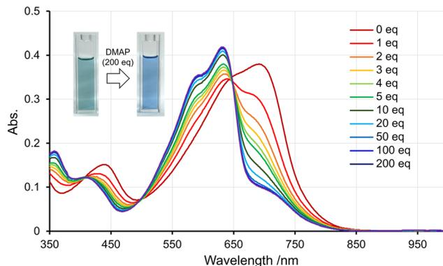
Fig. 5 UV-vis absorption data obtained from titrations of P2-HD with DMAP aliquots in CHCl<sub>3</sub> at the concentration of 0.01 mg mL<sup>-1</sup>. Insets show the response of P1-HD and P2-HD to the addition of DMAP.
