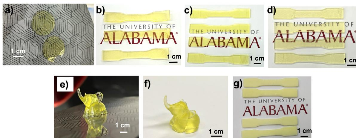
**Fig. 4** Photos of 3D printed samples: (a) poly(MAA-DMP) discs on the build plate (diameter: 20 mm, thickness 2 mm), (b) poly(MAA-DEP), (c) poly(MAA-DBP), (d) poly(MAA-DMEP), (e) and (f) 3D printed elephant from MAA-DEP monomer, and (g) poly(MAA-DEP)/PS10 printed as tensile bars ("dogbones" length: 82 mm, width: 12 mm, and thickness 2 mm).
