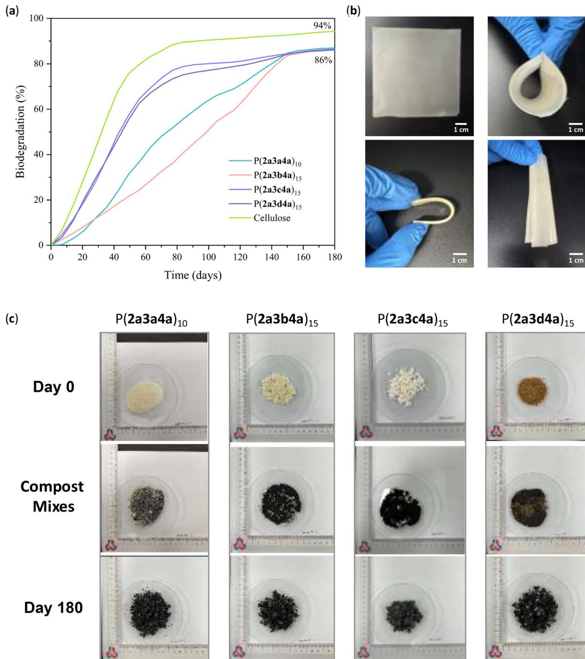
**Fig. 8** Illustration of the biodegradability of copolymers. (a) Experiment day versus biodegradation. (b) Photograph of a dumbbell-shaped specimen of P(2a3a4a)<sub>10</sub> under bending; photographs of a hot-pressed film (10 cm × 10 cm × 208 μm) and the film under bending. (c) Photographs from the composting degradation experiment for four polymers.
