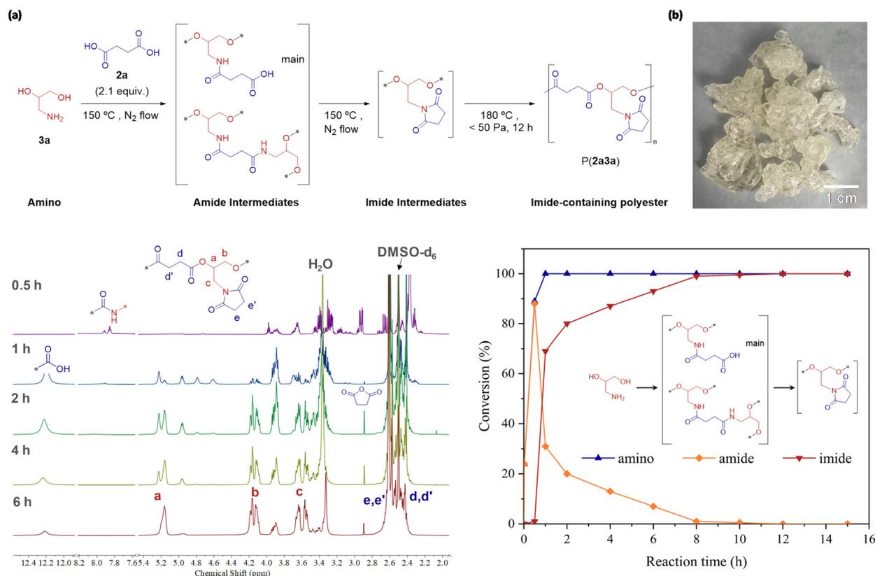
**Fig. 4** One-pot synthesis of imide-containing polyester P(**2a3a**) via conventional melt polycondensation. (a) Proposed reaction pathways. (b) Photograph of P(**2a3a**) as a transparent bulk solid. (c) Stacked <sup>1</sup>H NMR spectra of the reaction mixture at various time points. (d) Conversion kinetics from amino (**3a**) to amide to imide, quantified based on <sup>1</sup>H NMR data.
