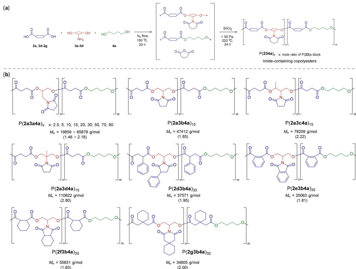
**Fig. 6** One-pot synthesis of imide-containing copolyesters from three-component starting materials. (a) Proposed reaction pathways. (b) The series of produced imide-containing copolyesters and corresponding molecular data.
