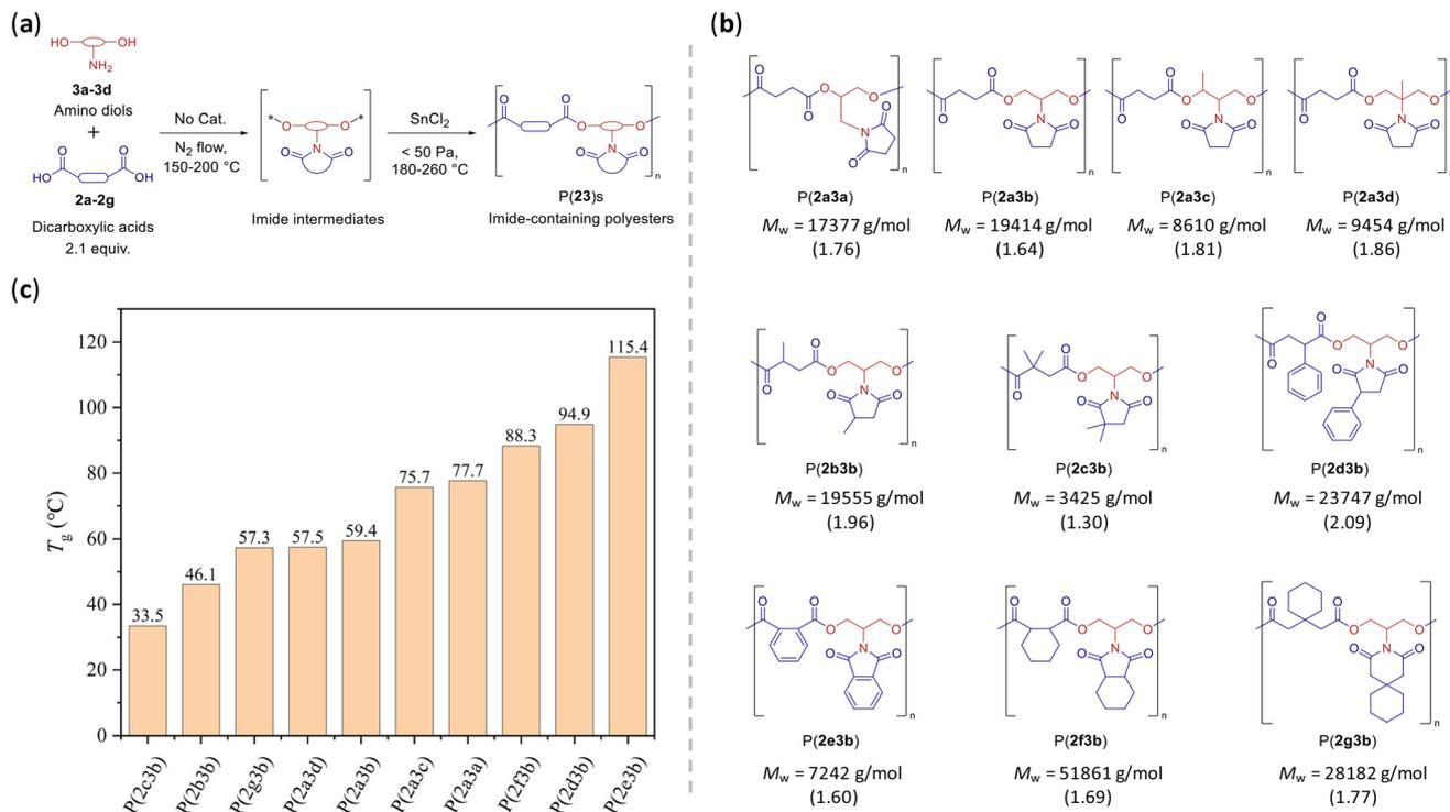
**Fig. 5** One-pot synthesis of imide-containing polyesters from two-component starting materials. (a) Proposed reaction pathways. (b) The series of produced imide-containing polyesters and corresponding molecular data. (c)  $T_g$  values of the imide-containing polyesters.
