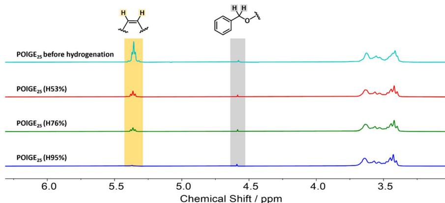
**Fig. 5** <sup>1</sup>H NMR spectra of POIGE<sub>25</sub> and the respective hydrogenated polymers (400 MHz, CDCl<sub>3</sub>). The value of *H* denotes the degree of hydrogenation. The intensity was locally normalized to the initiator benzyl group (gray).
