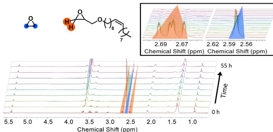
**Fig. 1** Stacked selection of  $^1\text{H}$  NMR spectra of the copolymerization of OIGE and EO. Zoom-in shows the decrease of the OIGE (orange) and EO monomer signals (blue). Polymerization temperature  $40\text{ }^\circ\text{C}$ , solvent:  $\text{DMSO-}d_6$  and  $\text{THF-}d_8$  1 : 5 (V/V), 400 MHz. As spectra were collected every 2 min for 55 h, only every 200th spectrum is displayed.
