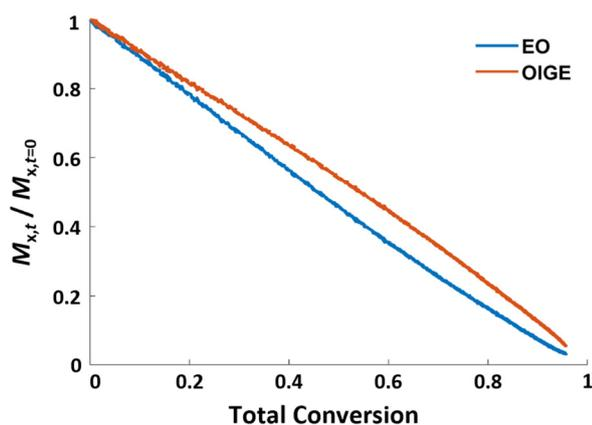
**Fig. 2** Unreacted monomer versus total conversion of the *in situ*  $^1\text{H}$  NMR copolymerization kinetic study of EO with OIGE. Solvent:  $\text{DMSO-}d_6/\text{THF-}d_8$  1 : 5 (V/V),  $40\text{ }^\circ\text{C}$ .
