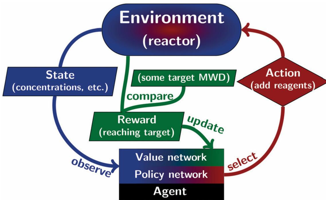
**Fig. 7** Reinforcement learning framework for optimizing molecular weight distribution (MWD) in atom transfer radical polymerization (ATRP). The AI agent observes the reaction state, selects actions (adjusting reagent addition), and updates its strategy based on real-time feedback and reward evaluation, iteratively improving polymerization outcomes. Reproduced with permission from ref. 87 Copyright 2018, Royal Society of Chemistry.
