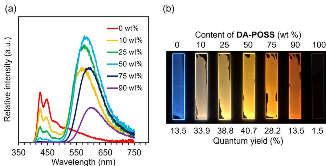
Fig. 3 (a) Relative photoluminescence spectra of PF and DA-POSS hybrid films excited at  $\lambda_{\text{abs, PF}}$  (385 nm). Numbers in the legend indicate the content ratios of DA-POSS. (b) Photos of PF and DA-POSS hybrid films irradiated by a UV lamp (365 nm).
