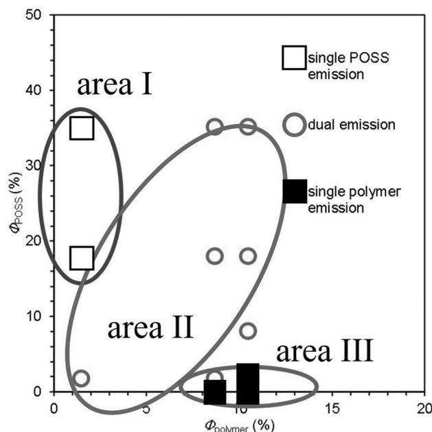
Fig. 2 Plots of the emission efficiencies of hybrid films containing POSSs. The horizontal and vertical axes represent  $\Phi_{\text{film,polymer}}$  and  $\Phi_{\text{film,POSS}}$ , respectively. The samples in area II showed dual emission from both the POSS and polymer. The samples in areas I and III showed emission from only the POSS or only the polymer, respectively.
