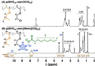
Fig. 2 <sup>1</sup>H NMR spectra of (A) p(IBVE-stat-CEVE) (in CDCl<sub>3</sub> at 30 °C; entry 4 in Table 1) and (B) p[IBVE-stat-([MeIm][C9])] (in DMSO-d<sub>6</sub> at 100 °C; entry 5 in Table 2). \*Grease, water, CHCl<sub>3</sub>, DMSO, Me<sub>4</sub>Si, etc.
