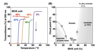
Fig. 4 (A) Turbidity measurement of (A)  $p[IBVE_n-stat-([MeIm][NA])_m]s$  in water (entries 1–5 in Table 4; polymer concentration: 2 wt%; scan rate = 1 °C min<sup>-1</sup>). (B) The relationship between solubility and thermoresponsivity in water of the statistical copolymers and IBVE content (the data are listed in Table 4, polymer concentration: 2 wt%).
