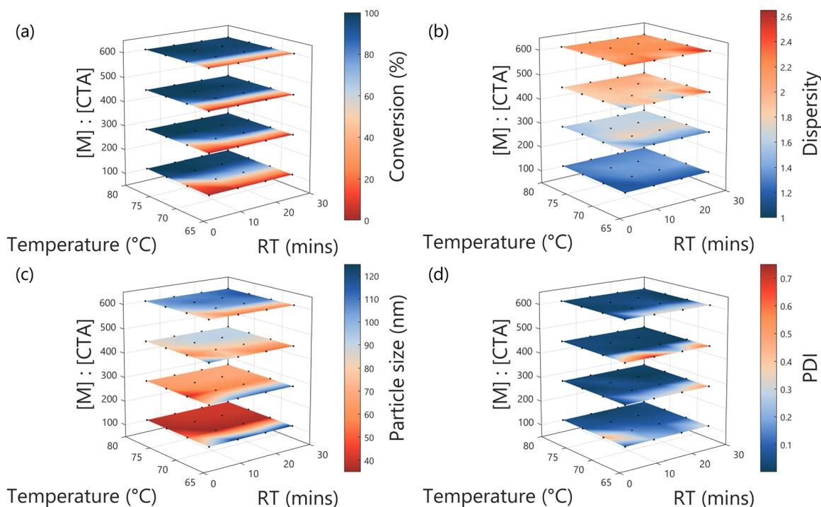
**Fig. 3** Results from the three-input full factorial DoE screen (temperature, residence time (RT) and monomer to CTA ratio ([M]:[CTA])), comprising 64 experiments, for (a) conversion, (b) molar mass dispersity, (c) particle size (nm) and (d) particle size PDI.
