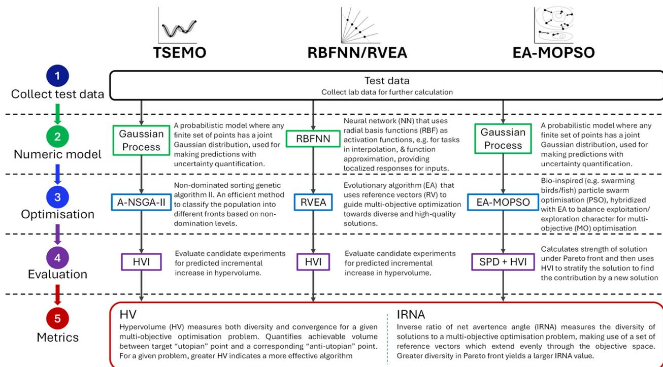
**Fig. 5** Summary of the optimisation strategies employed: Thompson sampling efficient multi-objective optimisation (TSEMO),<sup>11</sup> radial basis function neural network/reference vector evolutionary algorithm (RBFNN/RVEA) and multi objective particle swarm optimisation, hybridised with an evolutionary algorithm (EA-MOPSO).<sup>33</sup>
