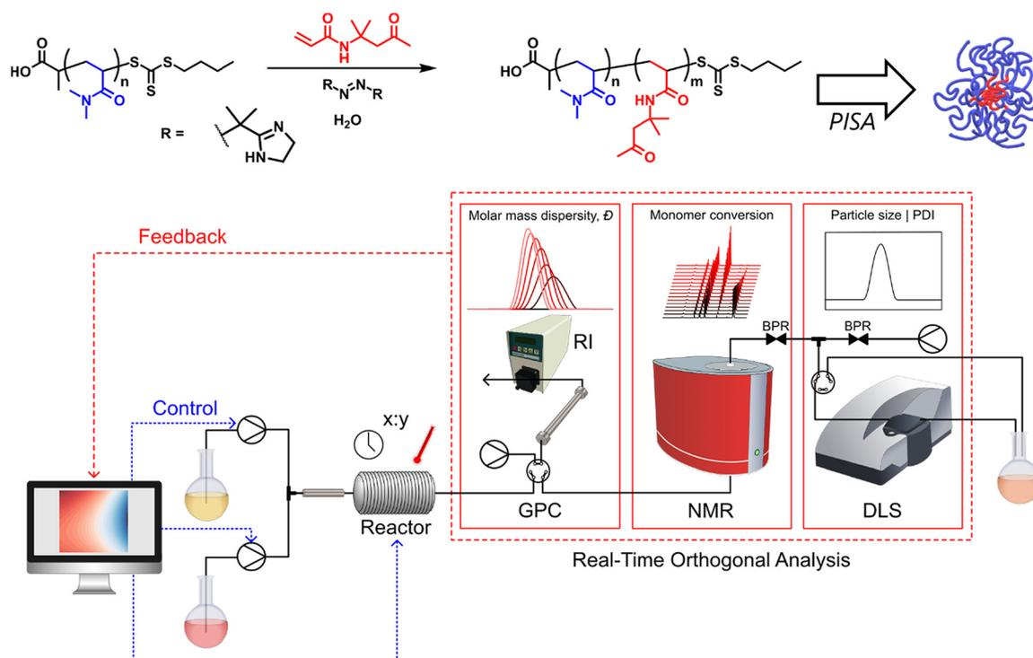
**Fig. 2** Overview of the chemistry and autonomous platform integrating a flow reactor and online gel permeation chromatography (GPC), <sup>1</sup>H nuclear magnetic resonance (NMR) spectroscopy and dynamic light scattering (DLS) used in this work.
