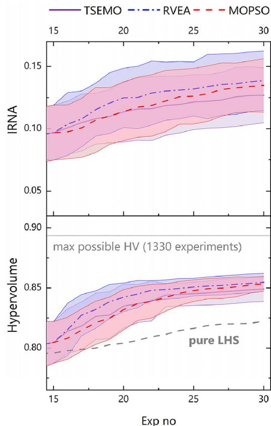
**Fig. 6** Mean evolution of hypervolume and inverse ratio of net average angle (IRNA) for the 20 optimisation campaigns for TSEMO, RBFNN/RVEA and EA-MOPSO. For hypervolume, the mean for 20 campaigns of 30 experiment Latin Hypercube sampling (LHS) of the decision space is also shown. The shaded area represents one standard deviation.
