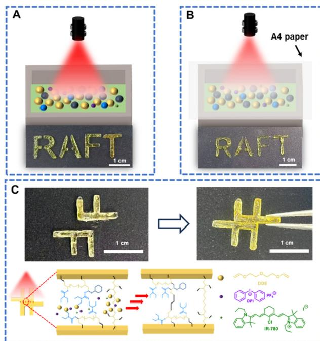
**Fig. 3** Photocuring using resin with a molar ratio of  $[DDE]_0/[CyVE]_0/[DTCB]_0/[DPI]_0/[IR-780]_0 = 70/30/1/0.5/0.01$  with a photomask under a 780 nm NIR light for (A) 1 minute and (B) 6 minutes with a A4 paper. (C) Polymer welding experiment.
