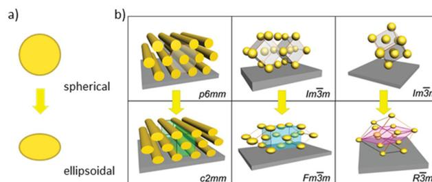
**Fig. 7** Effects induced by anisotropic shrinkage of the OMC film during carbonization, (a) distortion of the pore shape from spherical to ellipsoidal, (b) some examples of symmetry-allowed transitions of pore arrangements. (b) Reproduced from ref. 137 with permission from ACS, copyright 2025.
