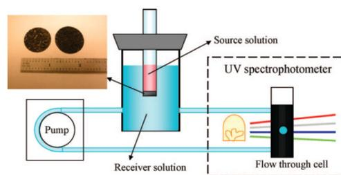
Fig. 16 Schematic setup used by Hou et al.<sup>176</sup> Reproduced from ref. 176 with permission from ACS, copyright 2025.
