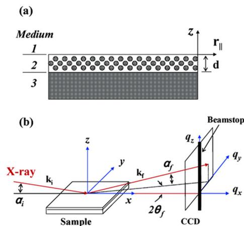
**Fig. 10** General GI-SAXS setup: (a) medium 1 = vacuum; medium 2 = mesostructured thin film with thickness  $d$ ; medium 3 = substrate with infinite thickness. (b)  $\alpha_i$  = incident angle;  $\alpha_r$  and  $2\theta_f$  = exit angles of the X-ray beam.  $k_i$  and  $k_r$  = wave vector of the incident and scattered X-ray beams.  $q_x$ ,  $q_y$ , and  $q_z$  = components of the scattering vector  $q$ . Reproduced from ref. 142 with permission from ACS, copyright 2025.
