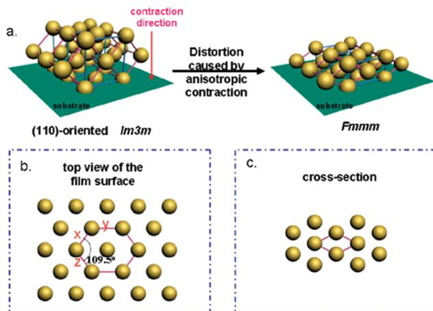
**Fig. 8** Illustration of (a) structural transformation of the OMC from  $Im3m$  to  $Fmmm$  symmetry during carbonization; distorted lattice from (b) the top and (c) cross-section. Reproduced from ref. 25 with permission from ACS, copyright 2025.
