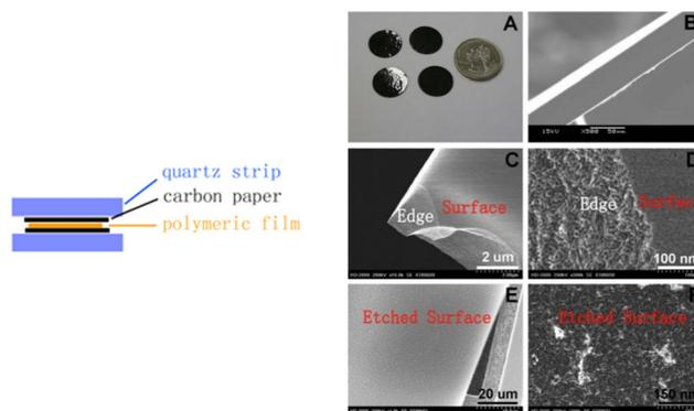
**Fig. 5** Left: Sandwich-type-carbonization. Right: Photograph (A) and cross-sectional SEM image (B) of the OMC film. STEM images of as-made (C and D) and surface-etched (E and F) OMC. Reproduced from ref. 35 with permission from Elsevier, copyright 2025.
