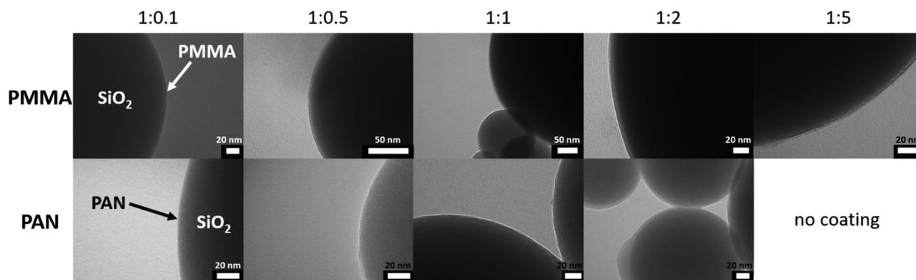
**Fig. 4** TEM micrographs of PMMA and PAN coatings on  $\text{SiO}_2$ -NPs at the respective monomer concentration in solution. Dark gray spherical shapes are the  $\text{SiO}_2$ -NPs with the lighter gray edges showing the amorphous polymer coating.
