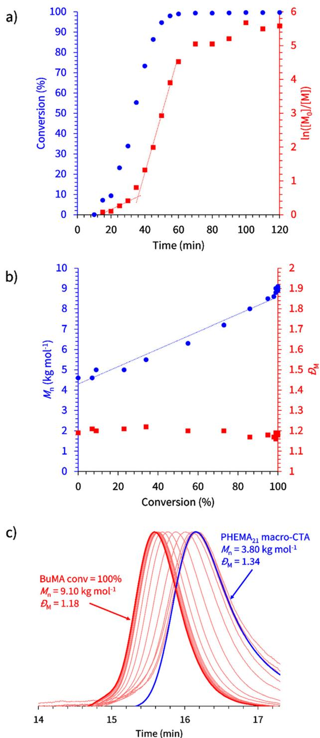
**Fig. 1** Kinetic study for the RAFT emulsion polymerisation of BuMA, targeting a degree of polymerisation of 100, in [EMIM][EtOSO<sub>3</sub>] at 10% w/w solids using a PHEMA<sub>21</sub> macro-CTA: (a) BuMA conversion vs. time (blue circles) and semi-log kinetic (red squares); (b)  $M_n$  (blue circles) and  $\bar{D}_M$  (red squares) vs. BuMA conversion; (c) DMF GPC chromatograms. GPC data were obtained against poly(methyl methacrylate) standards.
