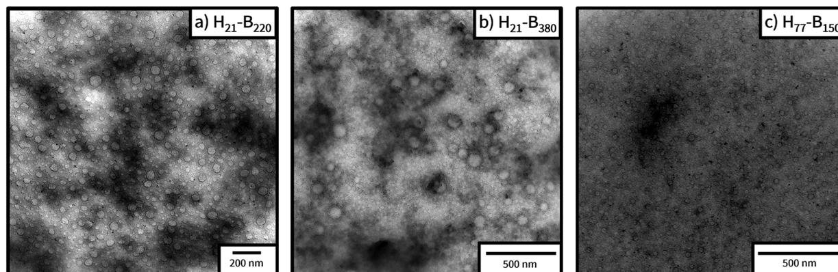
**Fig. 4** TEM images obtained for 0.10% w/w emulsions of PHEMA-*b*-PBuMA block copolymers prepared in [EMIM][EtOSO<sub>3</sub>].
