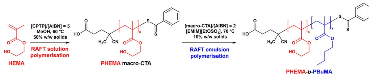
**Scheme 1** Synthesis of poly(2-hydroxyethyl methacrylate) (PHEMA) macro-CTA *via* RAFT solution polymerisation in methanol at 60 °C, followed by RAFT emulsion polymerisation of *n*-butyl methacrylate (BuMA) in 1-ethyl-3-methylimidazolium ethyl sulfate ([EMIM][EtOSO<sub>3</sub>]) at 70 °C to yield PHEMA<sub>*x*</sub>-*b*-PBuMA<sub>*y*</sub> diblock copolymers.
