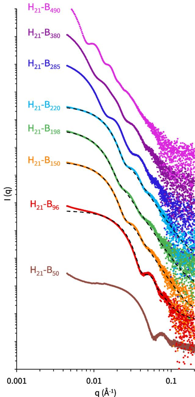
Fig. 5 Background-subtracted SAXS patterns recorded at 1.0% w/w for PHEMA<sub>21</sub>-*b*-PBuMA<sub>y</sub> spheres prepared via RAFT emulsion polymerisation, where dashed lines represent fits to the spherical micelle model. For clarity, data are offset on the y-axis by a factor of 10.
