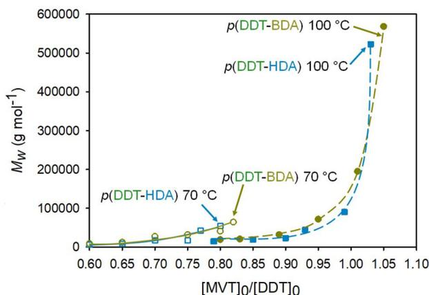
**Fig. 4** Variation in  $M_w$  for the diacrylate TBRT reactions conducted at 70 °C (BDA – yellow open circles; HDA – blue open squares) and 100 °C (BDA – yellow closed circles; HDA – blue closed squares) in the presence of DDT and varying  $[MVT]_0/[DDT]_0$  ratios.
