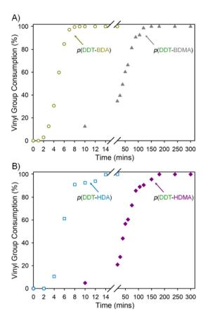
Fig. 2 Kinetic studies of the TBRT synthesis of (A) p(DDT-BDA) using  $[MVT]_0/[DDT]_0 = 0.80$  (open yellow circles) and p(DDT-BDMA) using  $[MVT]_0/[DDT]_0 = 0.67$  (grey triangles), and (B) p(DDT-HDA) using  $[MVT]_0/[DDT]_0 = 0.75$  (open blue squares) and p(DDT-HDMA) using  $[MVT]_0/[DDT]_0 = 0.65$  (purple diamonds).  $[MVT]_0/[DDT]_0$  ratios for this study were chosen as representative TBRT polymerisations unhindered by potential microgel formation.
