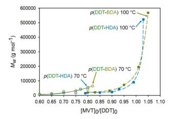
Fig. 4 Variation in  $M_{\rm w}$  for the diacrylate TBRT reactions conducted at 70 °C (BDA – yellow open circles; HDA – blue open squares) and 100 °C (BDA - yellow closed circles; HDA - blue closed squares) in the presence of DDT and varying [MVT]<sub>0</sub>/[DDT]<sub>0</sub> ratios.
