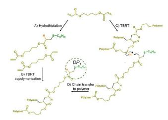
Scheme 2 Proposed mechanisms for the enhanced formation of  $DP_1$  structures within diacrylate TBRT. (A and B) Hydrothiolation leading to a mixed mono-/multi-vinyl taxogen feedstock and copolymerisation, and (C and D) conventional TBRT with additional chain transfer to polymer generating  $DP_1$  structures without the intervention of additional telogen.
