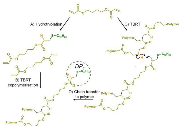
**Scheme 2** Proposed mechanisms for the enhanced formation of DP<sub>1</sub> structures within diacrylate TBRT. (A and B) Hydrothiolation leading to a mixed mono-/multi-vinyl taxogen feedstock and copolymerisation, and (C and D) conventional TBRT with additional chain transfer to polymer generating DP<sub>1</sub> structures without the intervention of additional telogen.
