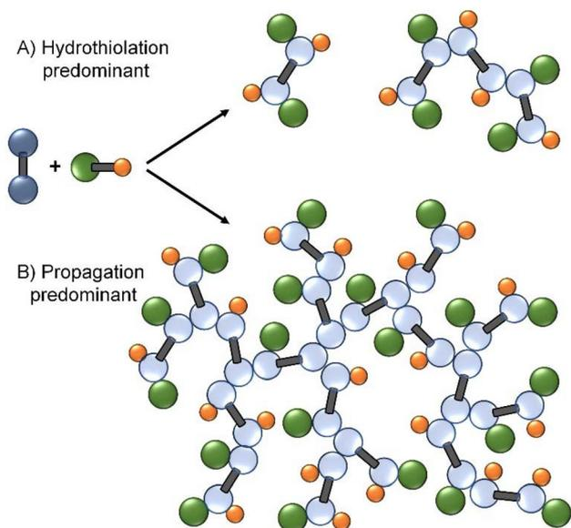
**Fig. 1** Schematic representations of possible outcomes of diacrylate TBRT: (A) hydrothiolation resulting from radical mediated thiol–ene addition, and (B) thiols acting as telogens under TBRT conditions and significant propagation.
