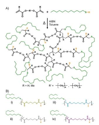
Scheme 1 TBRT synthesis of study branched polyesters. (A) General reaction scheme of multi-vinyl taxogens (diacrylate and dimethacrylate) with DDT; (B) nominal repeat unit structures detailing the synthesis of four branched polyesters *via* the TBRT of (i) BDA, (ii) BDMA, (iii) HDA and (iv) HDMA, with DDT utilised as the common telogen. Each polymer is shown as ideal (1:1) structures with pendant telogen residues.
