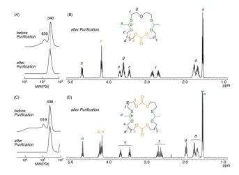
Fig. 1 SEC curves (A and C) and <sup>1</sup>H NMR spectra (CDCl<sub>3</sub>, r.t.) (B and D) of 22-CTAC (for A and B) and 26-CTAC (C and D) obtained by cationic thiol-ene reaction of DVE-1 and dithiols under dilute conditions:  $[DVE-1]_0/[DT-1]_0/[BSA]_0 = 25/25/0.10 \text{ mM or } [DVE-1]_0/[DT-2]_0/[BSA]_0 =$ 50/50/0.20 mM in CH<sub>2</sub>Cl<sub>2</sub> at -40 °C.
