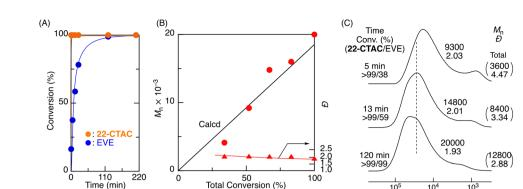
Fig. 2 Time-conversion curve (A),  $M_n$  values (B), and SEC curves (C) of the polymers obtained in cationic DT copolymerization of EVE and 22-CTAC:  $[EVE]_0/[22-CTAC]_0/[1]_0/[ZnCl_2]_0 = 4000/200/20/4.0 \text{ mM in CH}_2Cl_2/n-\text{hexane}/Et_2O (20/10/10) \text{ at } -40 ^{\circ}C.$
