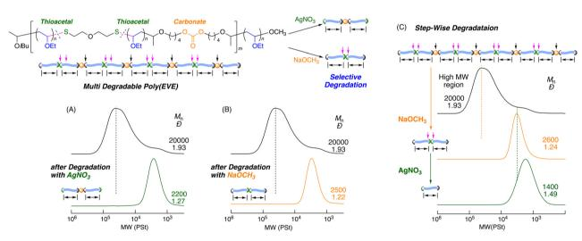
Fig. 4 SEC curves of the products before and after degradation with AgNO<sub>3</sub> (A) and NaOCH<sub>3</sub> (B), and SEC curves of the products obtained by dual degradation with the sequential use of NaOCH<sub>3</sub> and AgNO<sub>3</sub> (C): [thioacetal unit]<sub>0</sub>/[AgNO<sub>3</sub>]<sub>0</sub> = 5.0/50 mM in THF/H<sub>2</sub>O at 20 °C. [Carbonate]<sub>0</sub>/  $[NaOCH_3]_0 = 5.0/50$  mM in  $CH_3OH$  at 60 °C.
