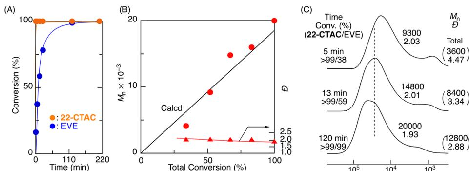
**Fig. 2** Time-conversion curve (A),  $M_n$  values (B), and SEC curves (C) of the polymers obtained in cationic DT copolymerization of EVE and 22-CTAC:  $[\text{EVE}]_0/[\text{22-CTAC}]_0/[\mathbf{1}]_0/[\text{ZnCl}_2]_0 = 4000/200/20/4.0$  mM in  $\text{CH}_2\text{Cl}_2/n\text{-hexane}/\text{Et}_2\text{O}$  (20/10/10) at  $-40$  °C.
