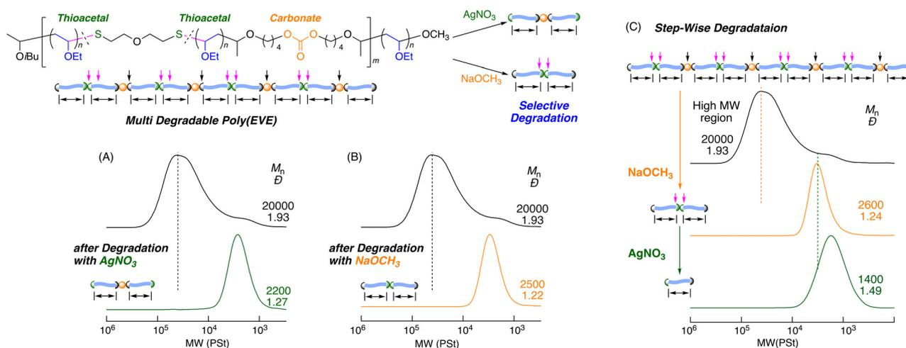
**Fig. 4** SEC curves of the products before and after degradation with  $\text{AgNO}_3$  (A) and  $\text{NaOCH}_3$  (B), and SEC curves of the products obtained by dual degradation with the sequential use of  $\text{NaOCH}_3$  and  $\text{AgNO}_3$  (C): [thioacetal unit] $_0$ /[ $\text{AgNO}_3$ ] $_0$  = 5.0/50 mM in  $\text{THF}/\text{H}_2\text{O}$  at 20 °C. [Carbonate] $_0$ /[ $\text{NaOCH}_3$ ] $_0$  = 5.0/50 mM in  $\text{CH}_3\text{OH}$  at 60 °C.
