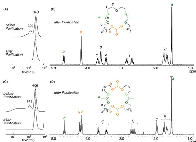
**Fig. 1** SEC curves (A and C) and  $^1\text{H}$  NMR spectra ( $\text{CDCl}_3$ , r.t.) (B and D) of 22-CTAC (for A and B) and 26-CTAC (C and D) obtained by cationic thiol-ene reaction of DVE-1 and dithiols under dilute conditions:  $[\text{DVE-1}]_0/[\text{DT-1}]_0/[\text{BSA}]_0 = 25/25/0.10 \text{ mM}$  or  $[\text{DVE-1}]_0/[\text{DT-2}]_0/[\text{BSA}]_0 = 50/50/0.20 \text{ mM}$  in  $\text{CH}_2\text{Cl}_2$  at  $-40^\circ\text{C}$ .
