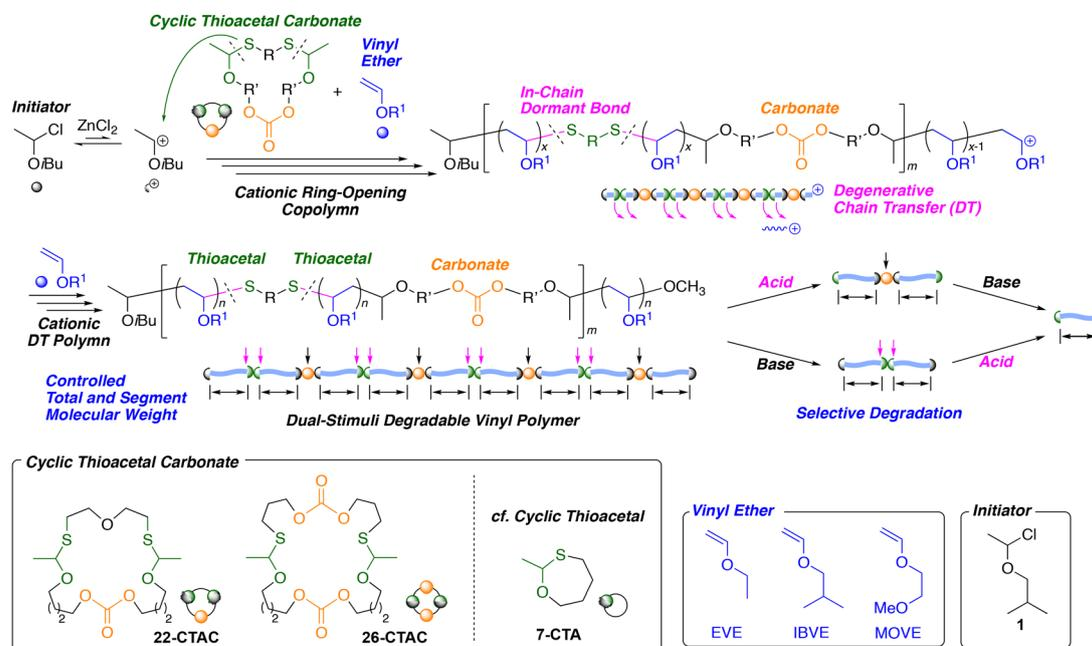
**Scheme 1** Synthesis and selective degradation of poly(vinyl ether)s with periodically distributed thioacetal and carbonate bonds in main chains by cationic degenerative chain-transfer copolymerization of vinyl ethers and cyclic thioacetal carbonate.
