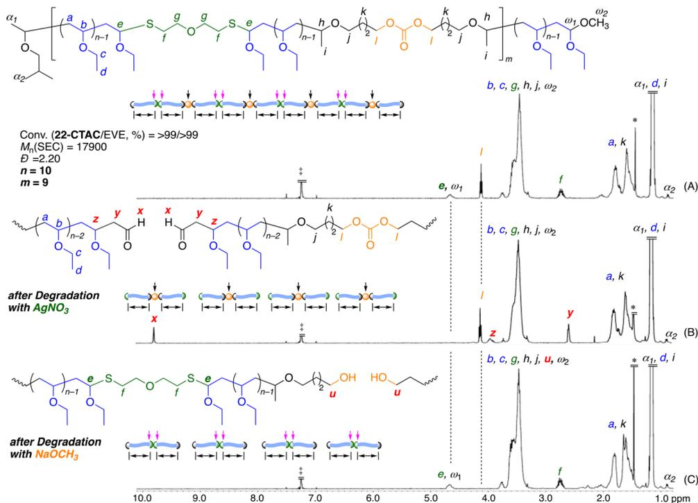
**Fig. 3**  $^1\text{H}$  NMR spectra ( $\text{CDCl}_3$ , 55 °C) of the obtained copolymer of EVE and 22-CTAC (A) and the polymers after degradation using an  $\text{AgNO}_3$  solution (B) and using a  $\text{NaOCH}_3$  solution (C): [thioacetal unit] $_0$ /[ $\text{AgNO}_3$ ] $_0$  = 5.0/50 mM in  $\text{THF}/\text{H}_2\text{O}$  at 20 °C or [carbonate unit] $_0$ /[ $\text{NaOCH}_3$ ] $_0$  = 5.0/50 mM in  $\text{CH}_3\text{OH}$  at 60 °C. \*:  $\text{H}_2\text{O}$ , †:  $\text{CHCl}_3$ .
