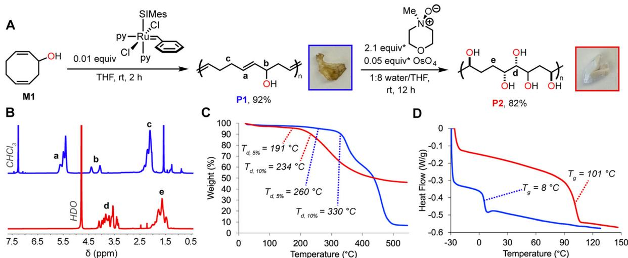
**Fig. 2** (A). Reaction scheme and photographs for synthesis of **P2**. Representative  $^1\text{H}$  NMR spectra (B), TGA (C), and DSC plots (D) for **P1** ( $10\text{ }^\circ\text{C min}^{-1}$ ;  $M_n = 86.7\text{ kg mol}^{-1}$ ) and **P2** ( $20\text{ }^\circ\text{C min}^{-1}$ ). \*Equivalents calculated and reported relative to **P1** repeat unit.
