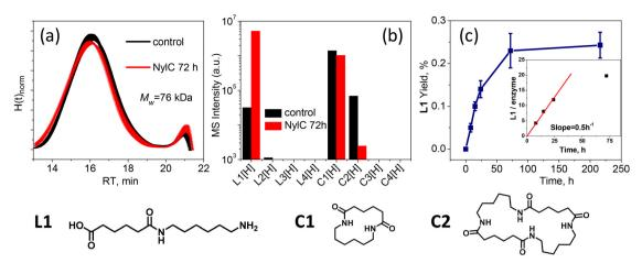
Fig. 1 Hydrolysis of washed commercial Nylon-6,6 by NylC. (a) Normalized SEC traces averaged over three biological replicates, with standard deviation (SD) included and (b) MS intensities for hydrolysis of commercial Nylon-6,6 incubated with (red) or without NylC (control, black) for 72 h. (c) L1 yield obtained from MS plotted vs. time. Inset: L1 to enzyme mole ratio for each kinetic point. The fitted line defines the linear regime of the reaction with the slope representing the reaction rate.
