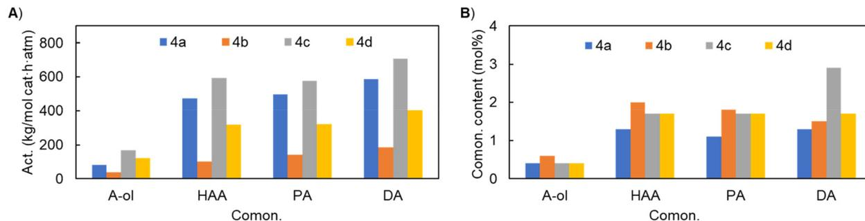
**Fig. 3** Effects of catalyst structures on ethylene copolymerization activity (A) and comonomer content (B) with various alkenol monomers (A-ol = allyl-OH; HAA = 3-buten-1-ol; PA = 4-penten-1-ol; and DA = 9-decen-1-ol).
