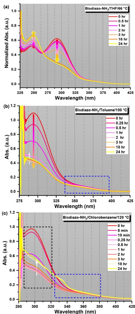
**Fig. 3** UV-vis kinetic traces of the polymerization of the bisdiazon-NH<sub>2</sub> compound in (a) THF as the solvent at 66 °C, (b) toluene at 100 °C and (c) chlorobenzene at 120 °C (concentration = 0.4 mg mL<sup>-1</sup>). UV-vis kinetic rate analysis: kinetic observation of the polymerization of bisdiazon-NH<sub>2</sub> in different solvent–temperature combinations using eqn (S11) and (S12).†
