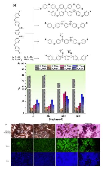
Fig. 1 (a) Chemical structures of bisdiazo-R compounds 1a-d and the possible repeating units of polymers under catalyst-free polymerization. (b) Elemental analysis and (c) optical and fluorescence images of bisdiazo-R compounds 1a-d with various terminal groups (R = H, Me, NO<sub>2</sub> and NH<sub>2</sub>).
