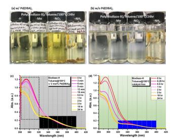
Fig. 6 (a and b) Images and (c and d) UV-vis kinetic spectra of polymer solutions in toluene at  $100\,^{\circ}\text{C}$  from the thermally induced polymerization of the bisdiazo-H compound (a and c) with (w/) and (b and d) without (w/o) the Pd(DBA)<sub>2</sub> catalyst.
