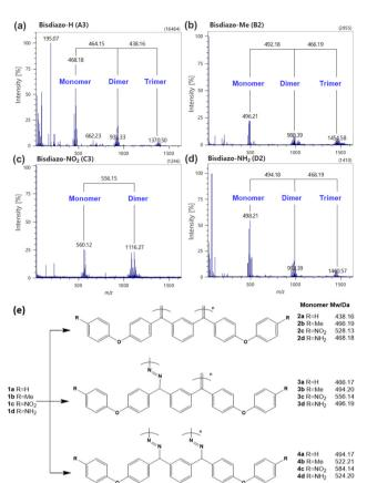
Fig. 7 FD HR-TOF MS spectra of the self-polymerized material upon heating under vacuum for (a) bisdiazo-H 1a, (b) bisdiazo-Me 1b, (c) bisdiazo-NO2 1c and (d) bisdiazo-NH2 1d; (e) possible repeating unit of oligomerization structures with monoisotopic m/z.
