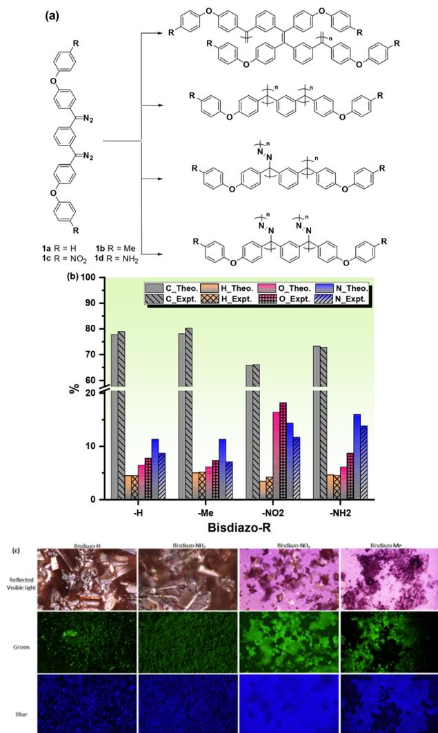
**Fig. 1** (a) Chemical structures of bisdiazon-R compounds **1a–d** and the possible repeating units of polymers under catalyst-free polymerization. (b) Elemental analysis and (c) optical and fluorescence images of bisdiazon-R compounds **1a–d** with various terminal groups ( $R = H, Me, NO_2$  and  $NH_2$ ).
