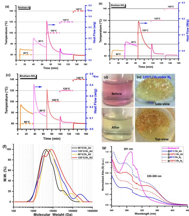
**Fig. 2** Stepwise isothermal DSC traces at various temperatures of (a) bisdiazio-H **1a**, (b) bisdiazio-NO<sub>2</sub> **1c** and (c) bisdiazio-NH<sub>2</sub> **1d**. (d) Colour change of bisdiazio-H solution in THF before and after heating, (e) self-polymerization in nitrogen at 120 °C for 3 h, (f) GPC traces of molecular weight distribution and (g) UV-vis spectra of self-polymerized bisdiazio-H **1a** under different conditions (in THF solution).
