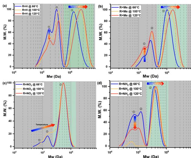
Fig. 5 GPC-obtained molecular weight (MW) distribution of bisdiazo-R polymerization in different solvent–temperature combinations for 24 h: (a) R = H, (b) R = Me, (c) R = NO<sub>2</sub> and (d) R = NH<sub>2</sub>.
