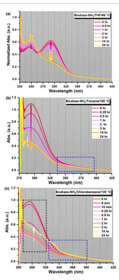
**Fig. 3** UV-vis kinetic traces of the polymerization of the bisdiazo-NH<sub>2</sub> compound in (a) THF as the solvent at 66 °C, (b) toluene at 100 °C and (c) chlorobenzene at 120 °C (concentration = 0.4 mg mL<sup>-1</sup>). UV-vis kinetic rate analysis: kinetic observation of the polymerization of bisdiazo-NH<sub>2</sub> in different solvent–temperature combinations using eqn (S11) and (S12).†
