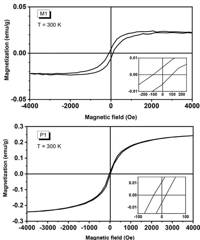
Fig. 3 The magnetization–magnetic field ( $M$ – $H$ ) curves of M1 crystals (upper) and P1 powders (lower) measured at 300 K. The saturation magnetization values for M1 and P1 are  $0.025$  and  $0.25 \text{ emu g}^{-1}$ , respectively. The insets show the magnified sections of the curves at around zero field.
