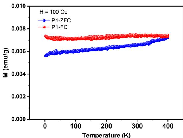
Fig. 4 Temperature-dependent magnetic properties of P1 powders: plots showing the variations in ZFC and FC magnetization intensity of P1 with temperature, measured at an applied magnetic field of 100 Oe.
