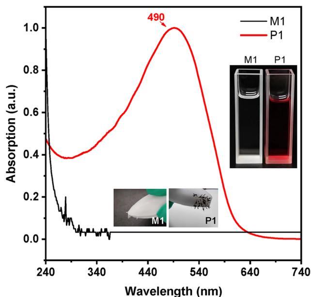
**Fig. 1** UV-visible absorption spectra of M1 and P1 in THF solution ( $1 \times 10^{-5}$  mol  $\text{L}^{-1}$ ). Inset photographs: right, M1 and P1 in THF solutions; bottom, powders of M1 and P1 adsorbed onto the surface of magnetic stir bars.
