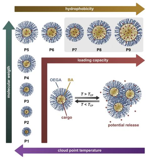
Fig. 5 Illustration of unimer size depending on amphiphilic balance and molecular weight in physiological salt solution at 37 °C with corresponding loading capacity for pyrene as drug proxy and thermally triggered aggregation into defined nanosized colloids due to their thermoresponsive properties. The most promising candidates for drug delivery applications P7–P9 are highlighted in grey.
