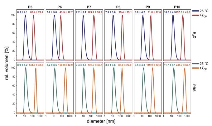
Fig. 4 Representative DLS curves of P(OEGA-co-BA) copolymers P5-P10 (10 mg ml<sup>-1</sup>) and their corresponding  $R_h$  below and above the respective  $T_{co}$  ( $T_{co}$  + 10 °C) in water and PBS. (n = 3).
