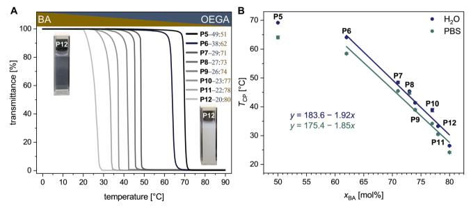
Fig. 3 (A) Representative normalised turbidity curves of P5–P12 in water determined at a heating rate of 0.5 °C min<sup>-1</sup> and a concentration of 10 mg mL<sup>-1</sup> with photographs of the aqueous solution of P12 below and above the phase transition temperature. (n = 3). (B) Plots of the measured cloud point temperature  $T_{cp}$  in water and PBS as a function of the average mole fraction of BA units per chain for the statistical P(OEGA-co-BA) copolymers.
