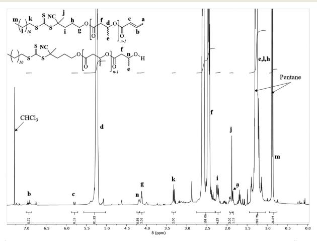
Fig. 1 <sup>1</sup>H NMR spectrum (500 MHz, CDCl<sub>3</sub>, 25 °C) of PHB<sub>83</sub>-TTC prepared by ROP of racemic β-butyrolactone catalyzed by Y{ONNO<sup>Me</sup><sub>1</sub>} in the presence of TTC-OH (Table 1, entry 1).
