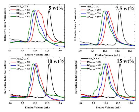
Fig. 5 SEC chromatograms (DMF, 25 °C) of PHB<sub>83</sub>-TTC macro-RAFT agent (black trace) and of the dispersions made at four different initial concentrations of HEMA *i.e.* 5 wt%, 7.5 wt%, 10 wt% and 15 wt% for different targeted degrees of polymerization, DP = 200 (red trace), 350 (blue trace) and 500 (green trace).
