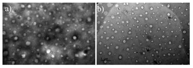
Fig. 7 TEM micrographs of PHB<sub>83</sub>-b-PHEMA<sub>500</sub> made at (a) 5 wt% and (b) 7.5 wt% of HEMA comonomer and PHB<sub>83</sub>-TTC macro-RAFT agent
