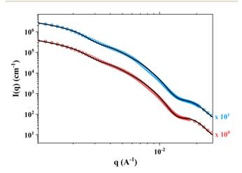
Fig. 8 SAXS patterns of PHB<sub>83</sub>-b-PHEMA<sub>500</sub> prepared at 5 wt% (in red) and 7.5 wt% (in blue) of HEMA comonomer and PHB<sub>83</sub>-TTC macro-RAFT agent concentration. The data fits obtained by using a spherical vesicle model is shown in black solid lines. The I(q) profiles were multiplied by a constant indicated on the Figure, so as to improve its readability.
